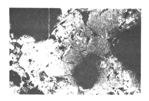
PLATE 2: Micrograph of a polished specimen of the same Heybridge slag. The major phases present are: Fayalite - light grey faceted phase Iron Oxide - white rounded phase. The glassy matrix occurs between some of the fayalite crystals. The black areas are voids. (magnification x 54).
