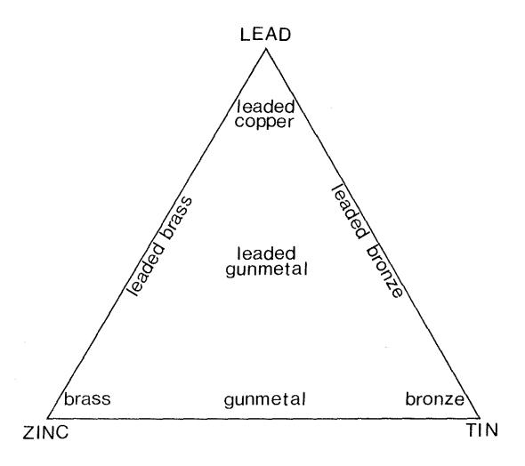
Figure 1 - The composition of copper alloys
