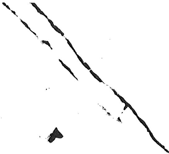
Plate XII Slag Inclusion (single phase) SEM Electron Image
