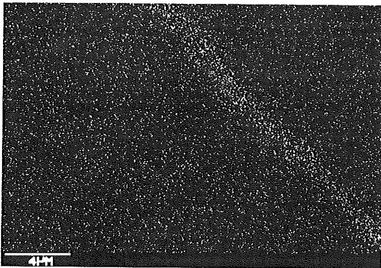
Plate XIII Slag Inclusion (single phase) Si Distribution
