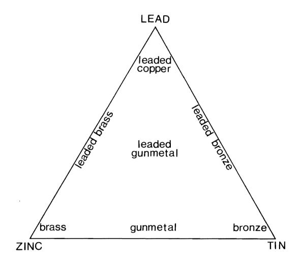
Figure 1: Composition of copper alloys
