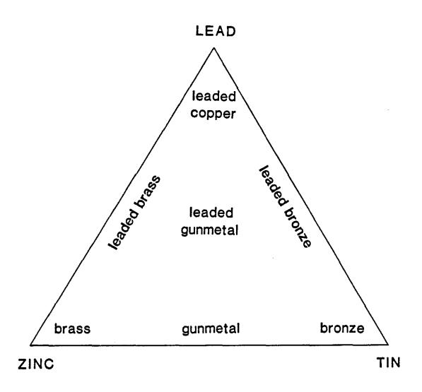
Figure 1: Ternary diagram showing the names applied to alloys of different compositions
