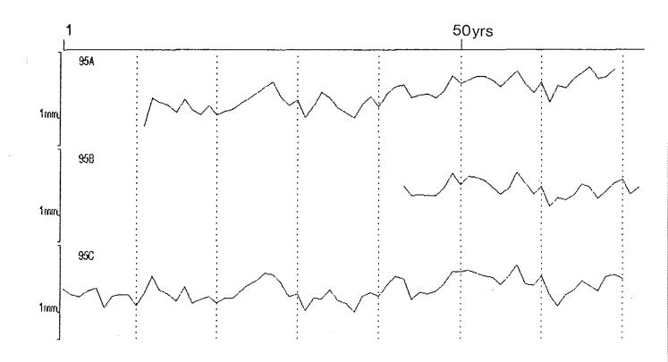
Fig 3: Matching ring sequences from the churn dash. <u>95A</u> - curved crosssectional measurements from the top of the artifact; <u>95B</u> - ring measurements along the short cross-sectional break from edge to centre; <u>95C</u> - measurements along the longitudinal grain.
