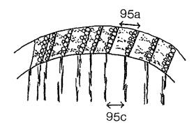
Fig 2: Schematic drawing of the wood structure on the churn dash. Arrows denote the boundaries of the same annual growth ring in cross-section (top) and longitudinal section (bottom).
