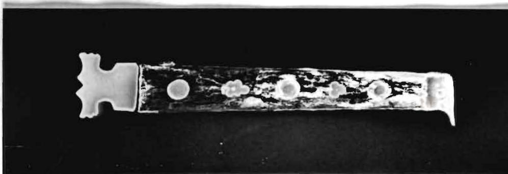
Figure 14: Negative xeroradiograph of knife handle from Hinton Hall Haddenham. 70kV 5mA 20 seconds (A&C)/70kV 5mA 30 seconds (B&D).
