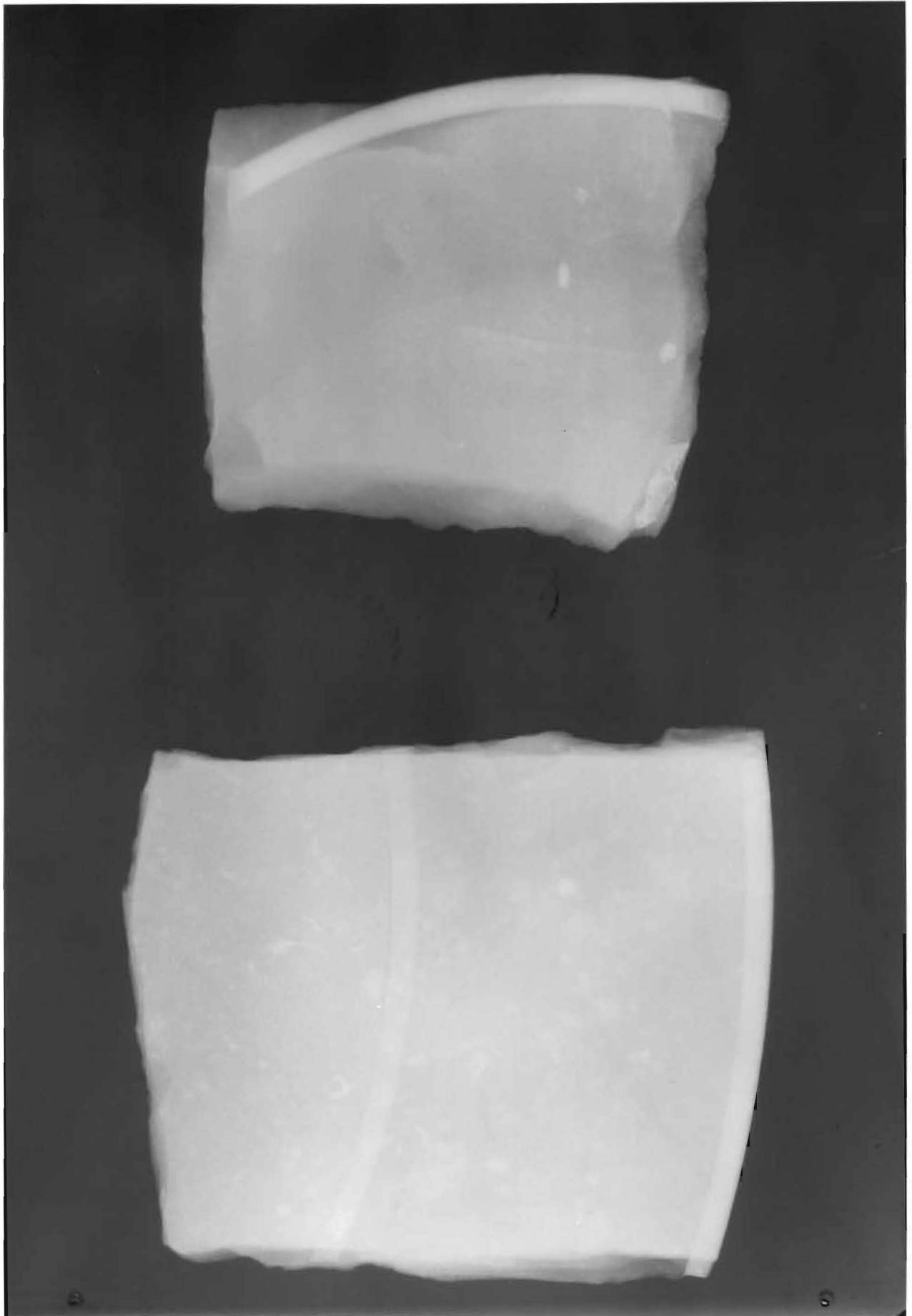
Figure 17: Film radiograph of shale platters from the Museum of London. 30kV 5mA 90 seconds.
