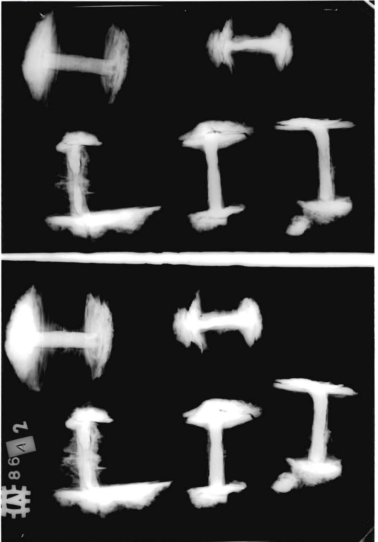
Figure 9: Film radiograph of coffin nails from York Minster. 80kV 5mA 40 seconds/90kV 5mA 60 seconds.
