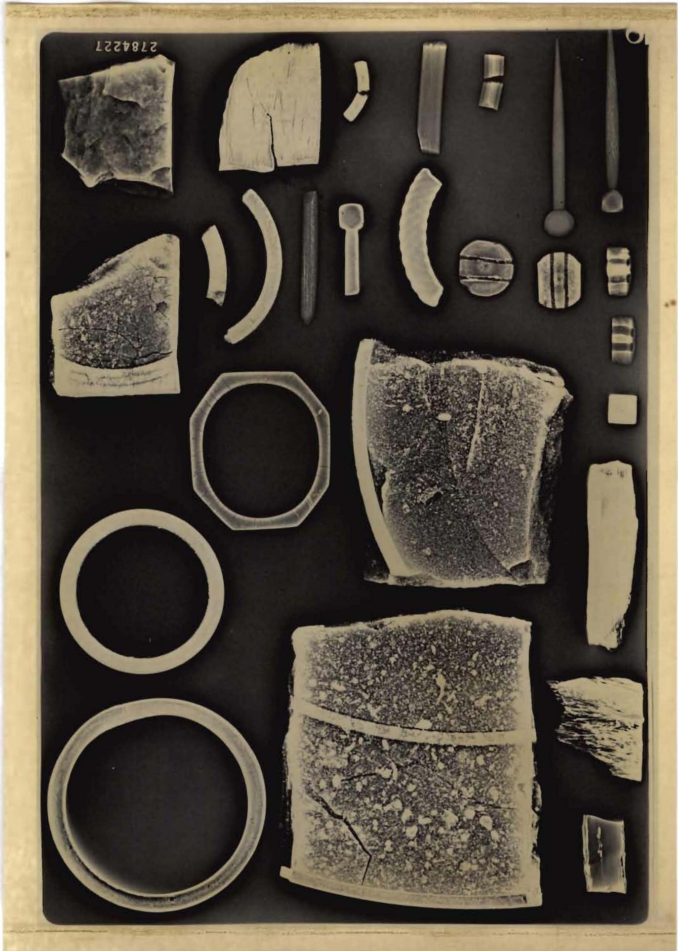
Figure 21: Negative xeroradiograph of jet/shale from various sites.
