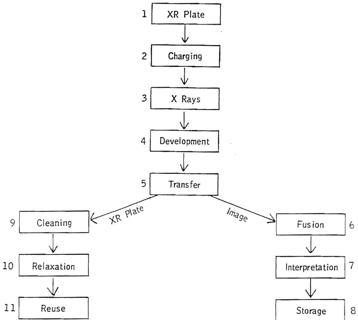
Figure 2: Flow chart of the various stages in the xeroradiography process.
