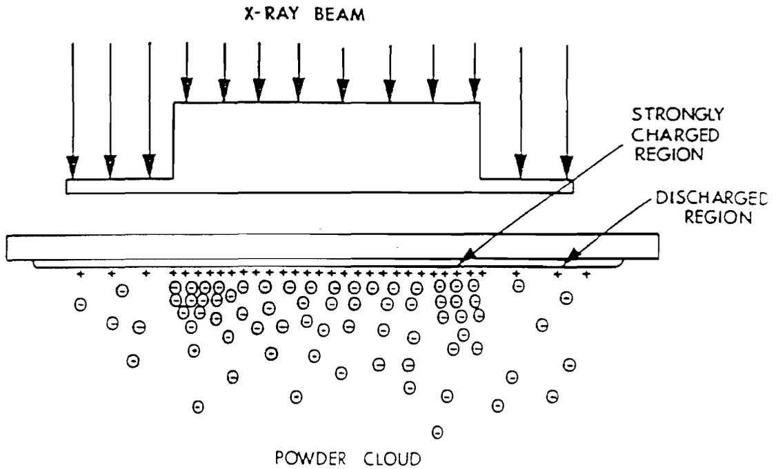
Figure 3: The charged powder is attracted to areas where the x-ray beam has been prevented from dissipating the charge on the plate. Concentrations of powder build up at the interfaces between areas of high and low charge.
