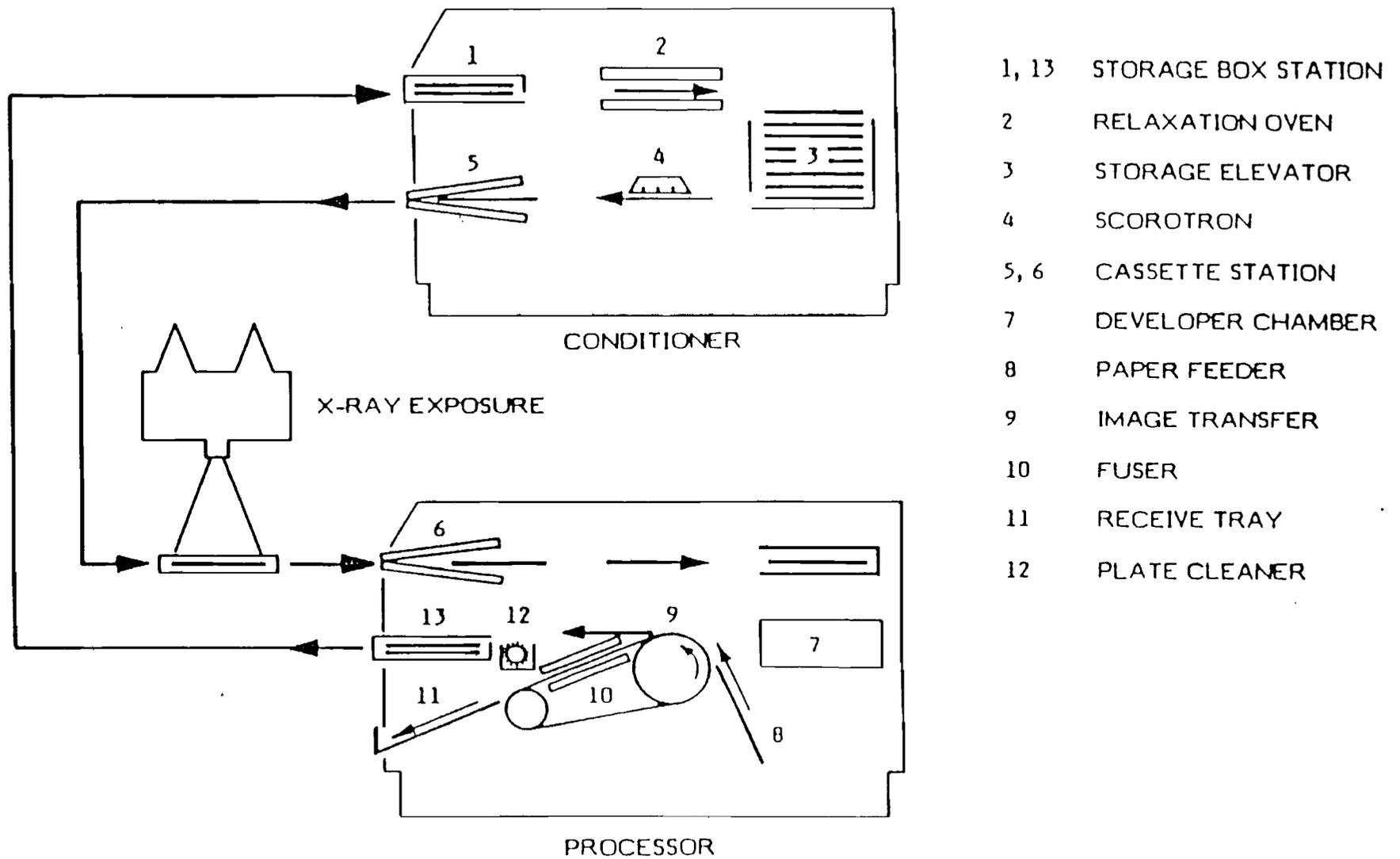
Figure 1: Schematic diagram of xeroradiographic equipment.
