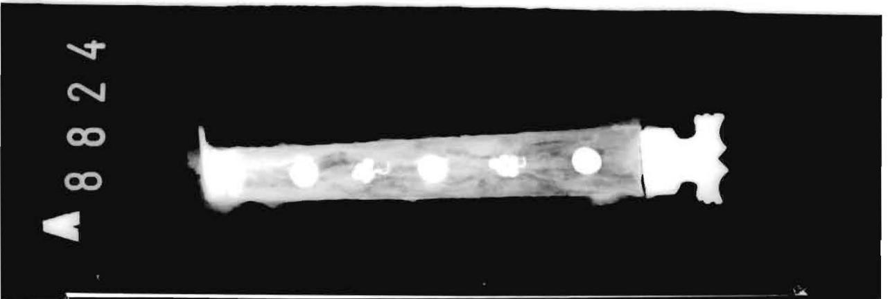
Figure 12: Film radiograph of knife handle from Hinton Hall Haddenham. 70kV 5mA 20 seconds (A&B)/70kV 5mA 30 seconds (C&D).
