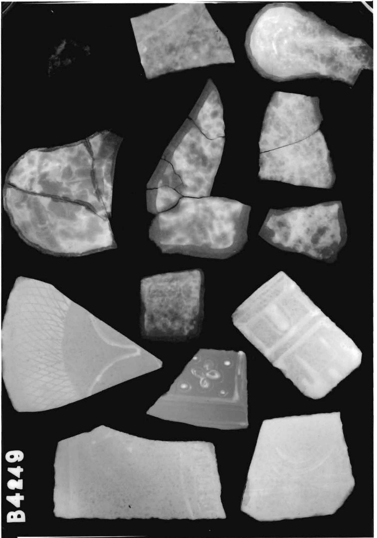
Figure 5: Film radiograph of medieval window glass from Bayham Abbey and Denny Abbey. 30kV 10mA 50 seconds.
