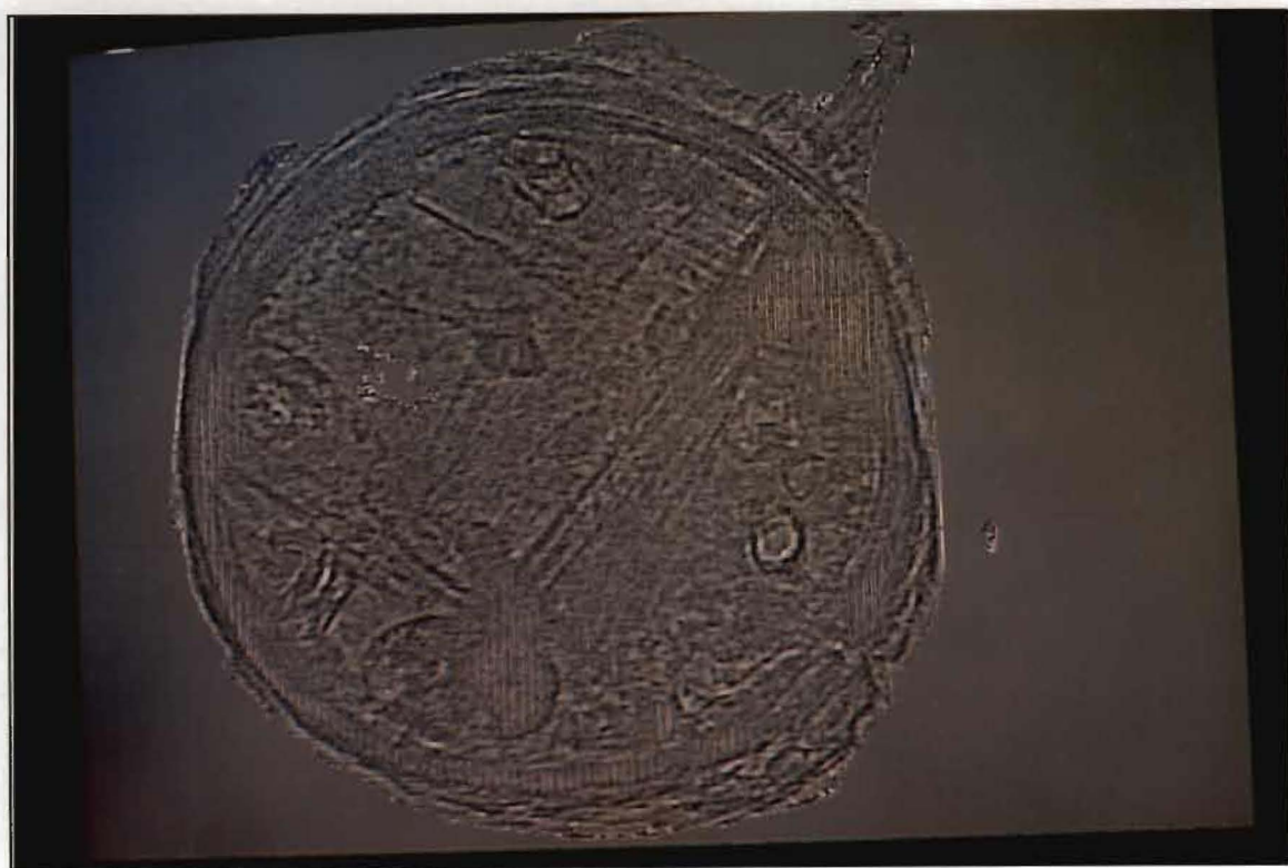
Figure 51 The effects of a Laplacian filter. Note that the areas of poor digitisation i.e. the vertical lines are particularly visible.
