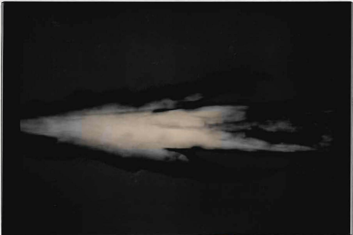
Figure 39 Original radiograph of iron arrowhead. The background has been masked to grey using the LUT in figure 9. The histogram of the grey levels is illustrated in figure 22.
