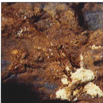
Figure 4. Cross section of wood preserved on iron staple. (Mag c.8x. WILD 85:4)
