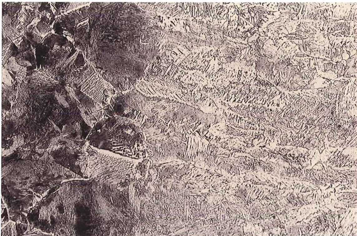
Plate 9 Garrison Church gate. Micrograph etched x200 Left: heat affected zone to left, Right: weld metal with widmanstätten structure
