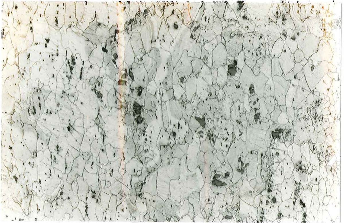
Plate 3: Ferrite grains. Etched, 250x magnification, Norbury Park.
