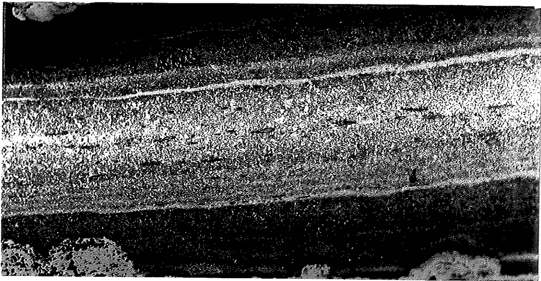
Plate 5. Knife \Delta 404 (980003). Centre of blade, with cutting edge to the left, showing banded structure comprising mainly martensite (darkly etching) and bainite (lighter etching). X100. Nital etch
