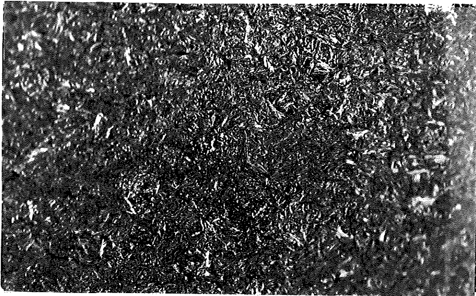
Plate 7. Knife Δ434 (980004). Martensite at the cutting edge. X200. Nital etch
