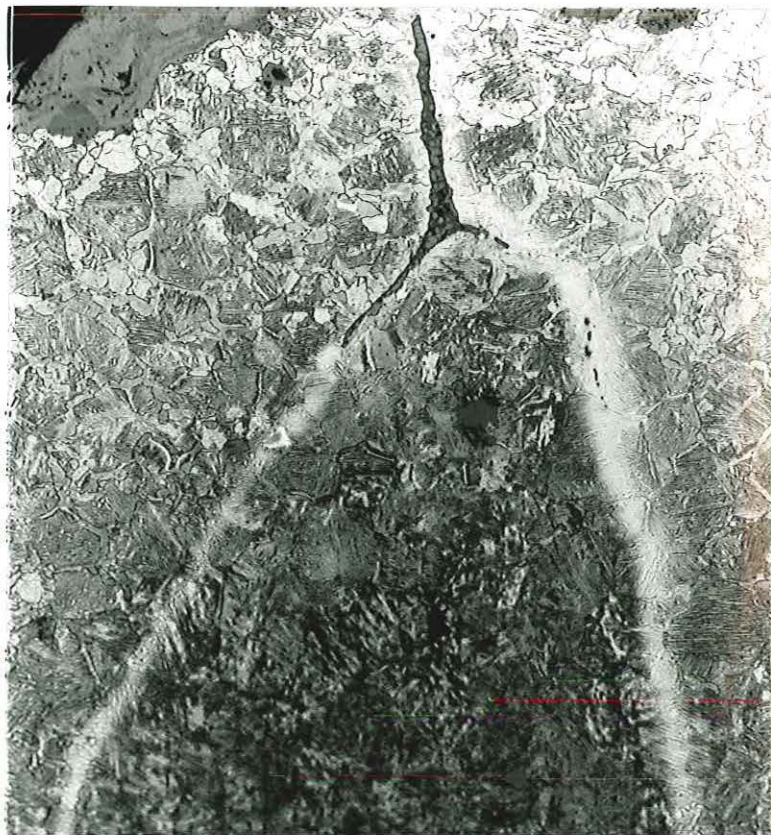
Plate 2. Knife \Delta 158 (980001). Detail: martensite (dark), with weld lines (white) and dual-phase inclusions at centre top weld. X100. Nital etch
