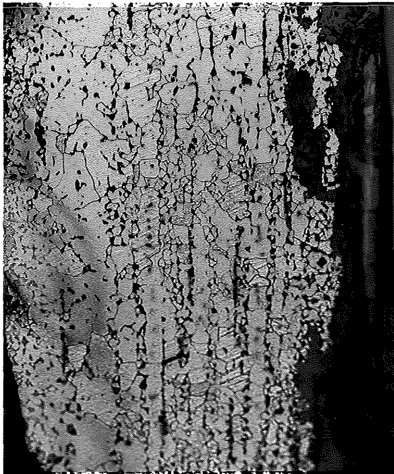
Plate 10. Knife Δ1242 (980006). Banded structure towards the cutting edge (orientated at the base) comprising mainly ferrite. X100. Nital etch
