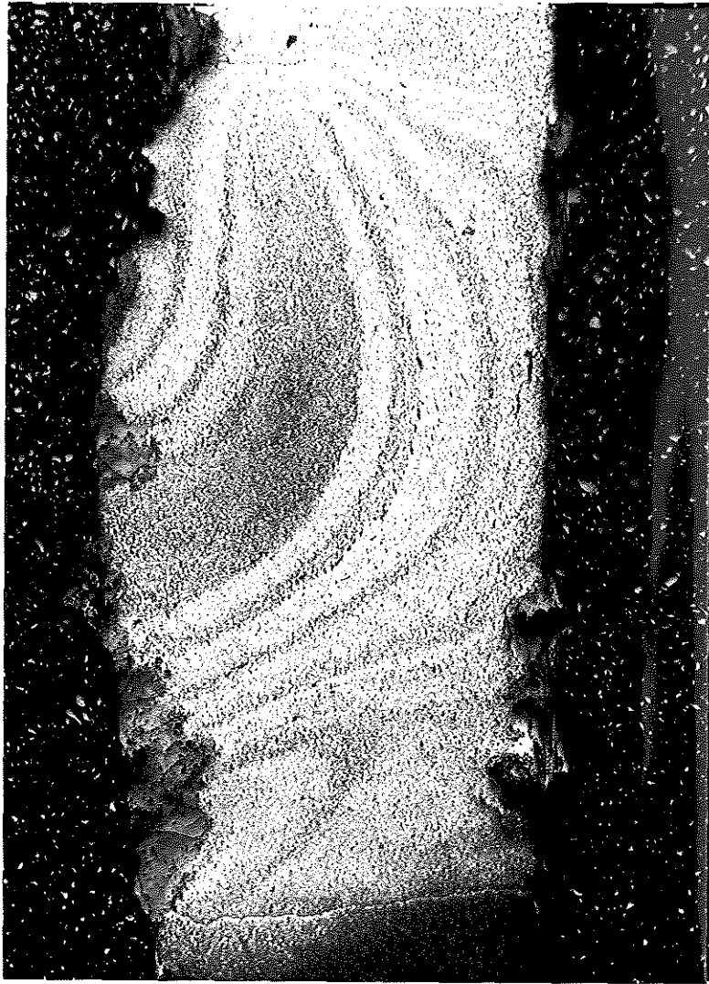
Plate 3. Knife Δ209 (980002). Pattern-welded zone at blade centre, the bands formed of variable carbon content, the darker etching areas containing more carbon. X50. Nital etch
