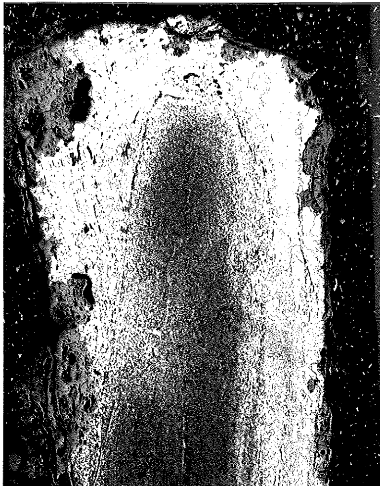
Plate 8. Knife Δ816 (980005). Blade back (at top). Ferrite (light etching) was wrapped around a core (darker etching) of higher-carbon content comprising martensite and pearlite. X50. Nital etch
