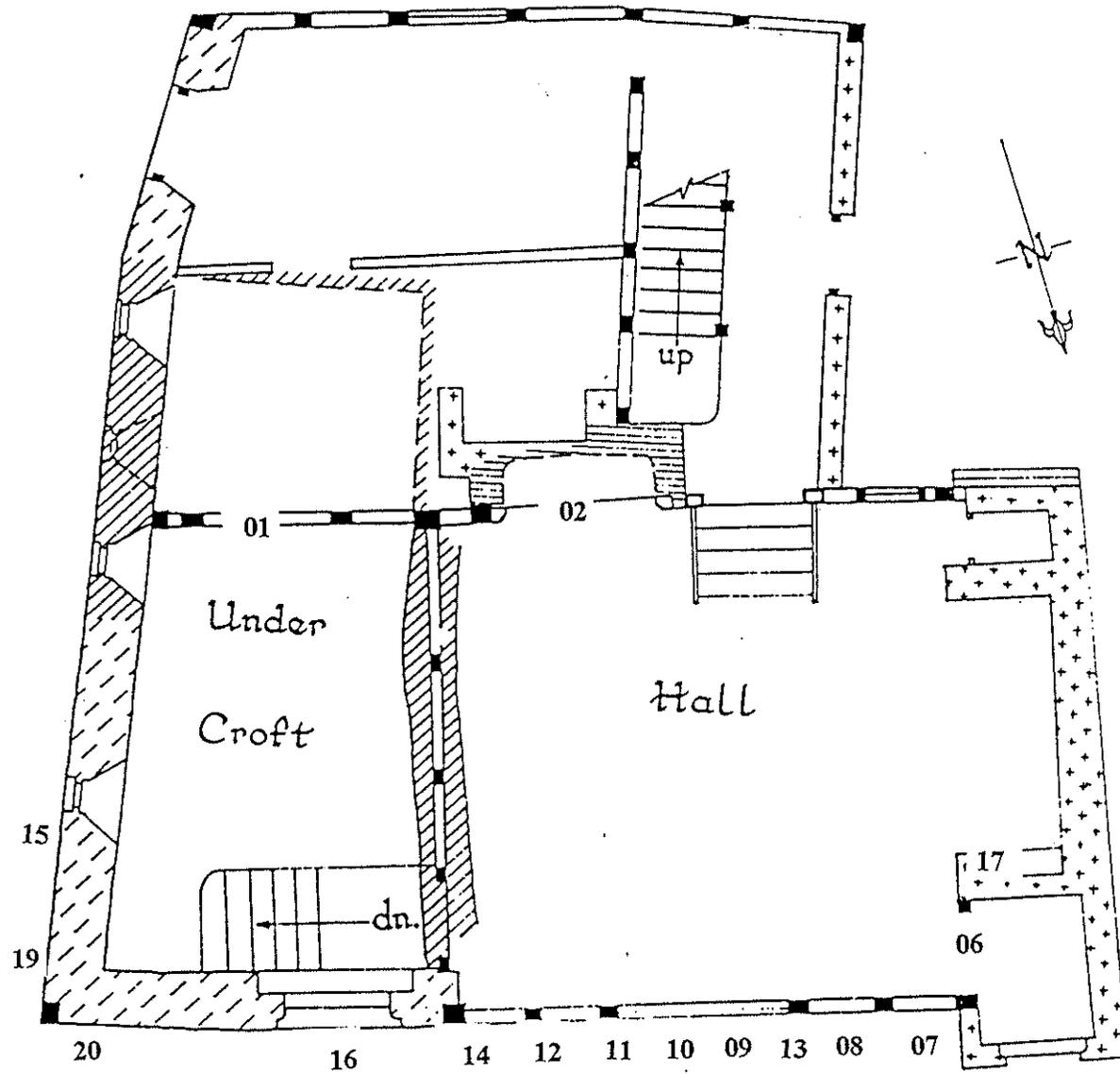
Figure 4b: Plan of first floor to show sample locations
