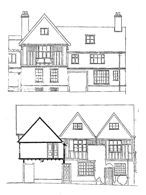
Figure 4: Front (upper) and side (lower) elevations of Nos 80 and 80A Fore Street, Ipswich
