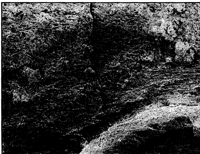
Figure 2. Detail of the iron corrosion on knife tang sf. 7162/3, in which a platelet structure can clearly be seen.
