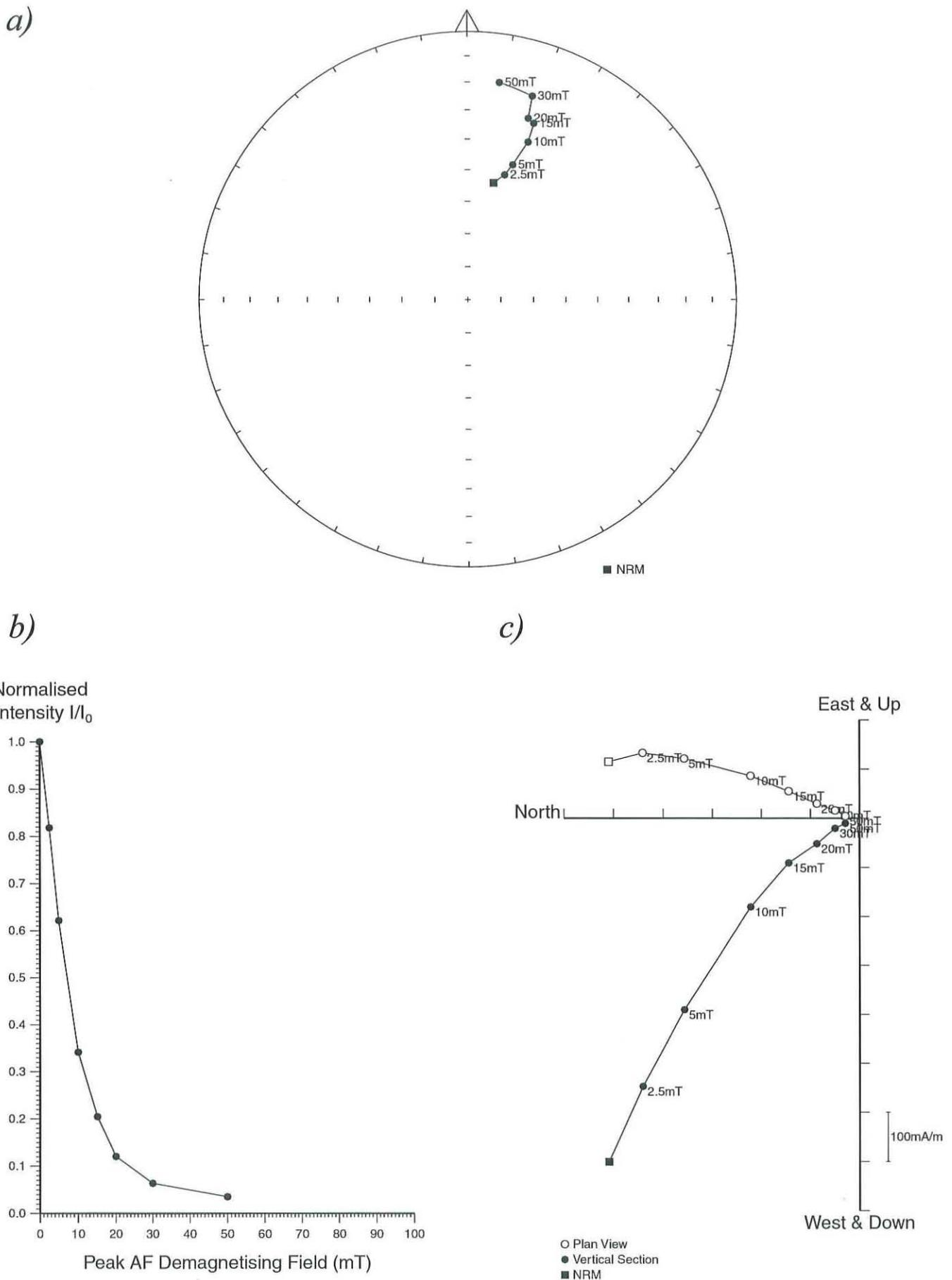
Figure 3: Stepwise AF demagnetisation of sample WD10. Diagram a) depicts the variation of the remanent direction as an equal area stereogram (declination increases clockwise, while inclination increases from zero at the equator to 90 degrees at the centre of the projection); b) shows the normalised change in remanence intensity as a function of the demagnetising field; c) shows the changes in both direction and intensity as a vector endpoint projection.
