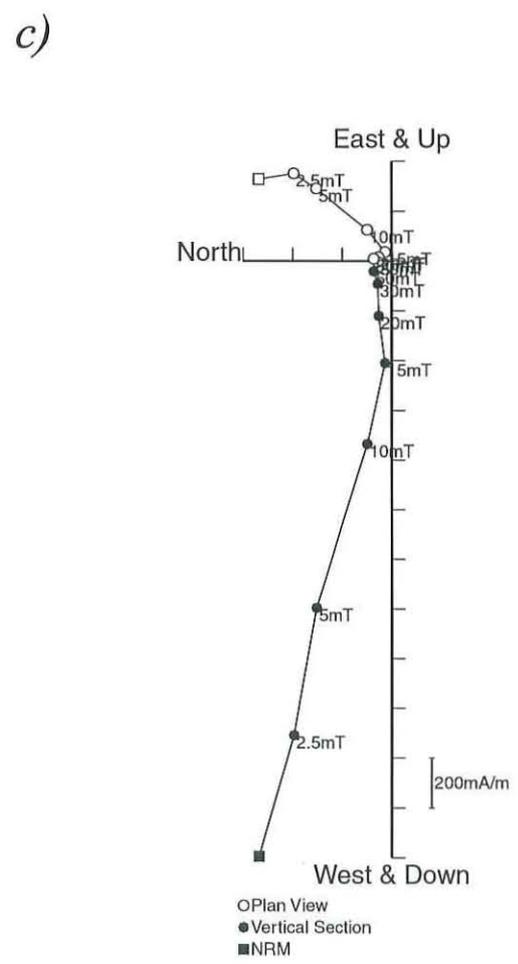
Figure 4: Stepwise AF demagnetisation of sample WD13. Diagram a) depicts the variation of the remanent direction as an equal area stereogram (declination increases clockwise, while inclination increases from zero at the equator to 90 degrees at the centre of the projection); b) shows the normalised change in remanence intensity as a function of the demagnetising field; c) shows the changes in both direction and intensity as a vector endpoint projection.
