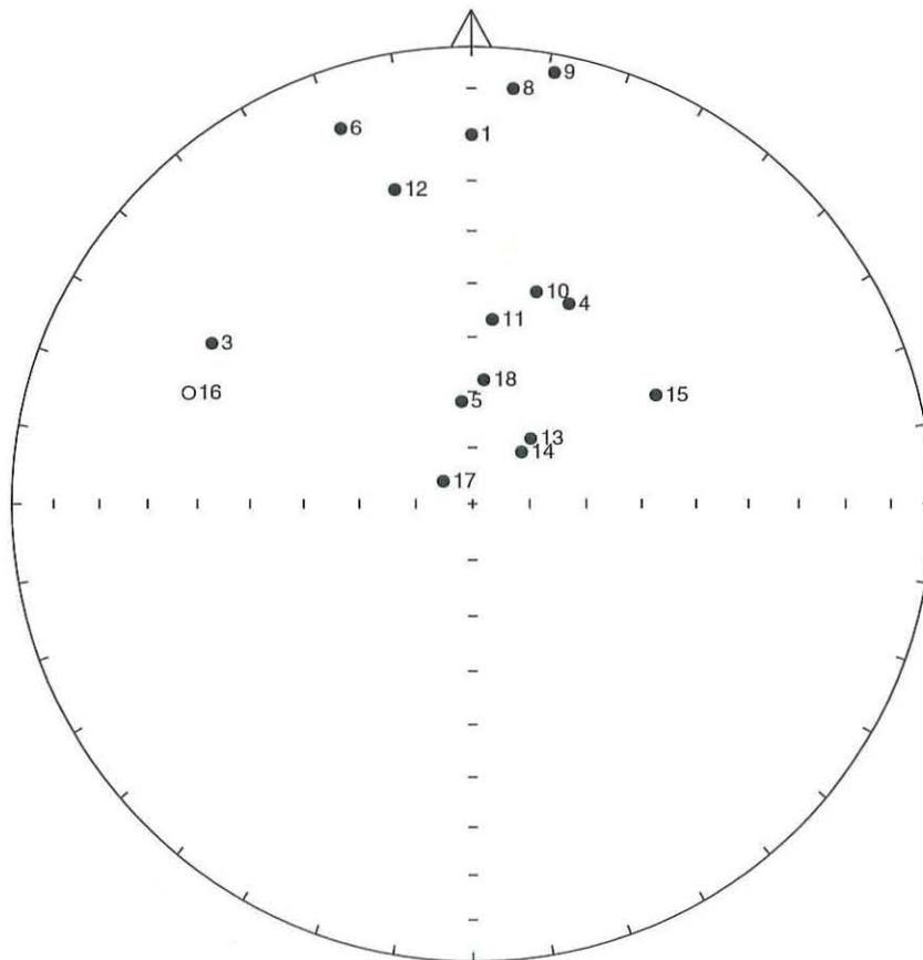
Figure 1: a) Distribution of NRM directions of samples from West Denton represented as an equal area stereogram. In this projection declination increases clockwise with zero being at 12 o'clock while inclination increases from zero at the equator to 90 degrees in the centre of the projection. b) Distribution of thermoremanent directions of magnetisation of the same samples after partial AF demagnetisation to 2.5mT.
