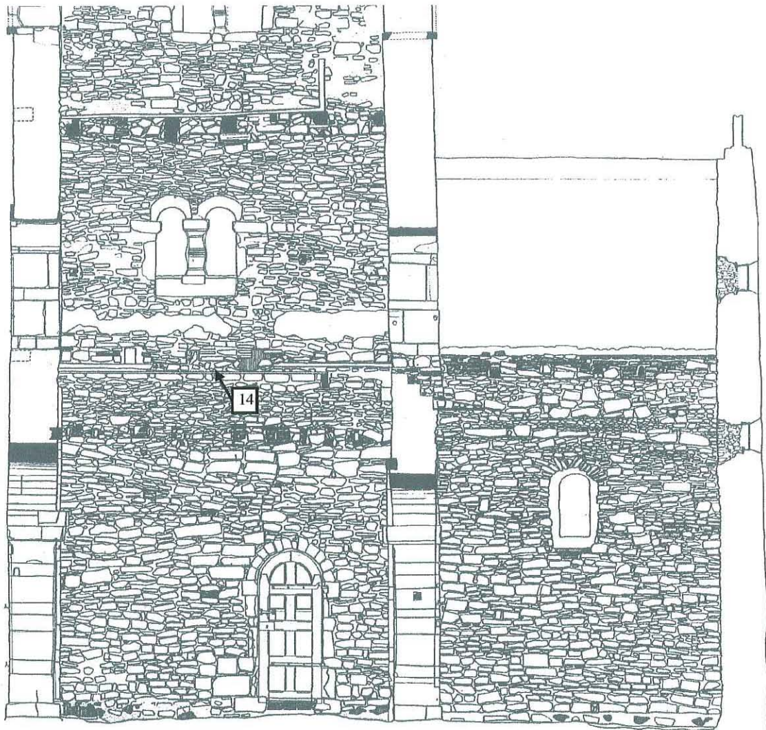
Figure 5 Internal elevation of the south walls of the lower part of the tower and baptistry (after Atkins and Rodwell pers comm), showing approximate location of samples from this area
