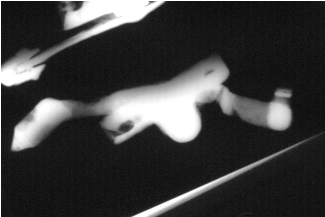
Figure 5: X-radiograph showing broken end of articulated terminal
