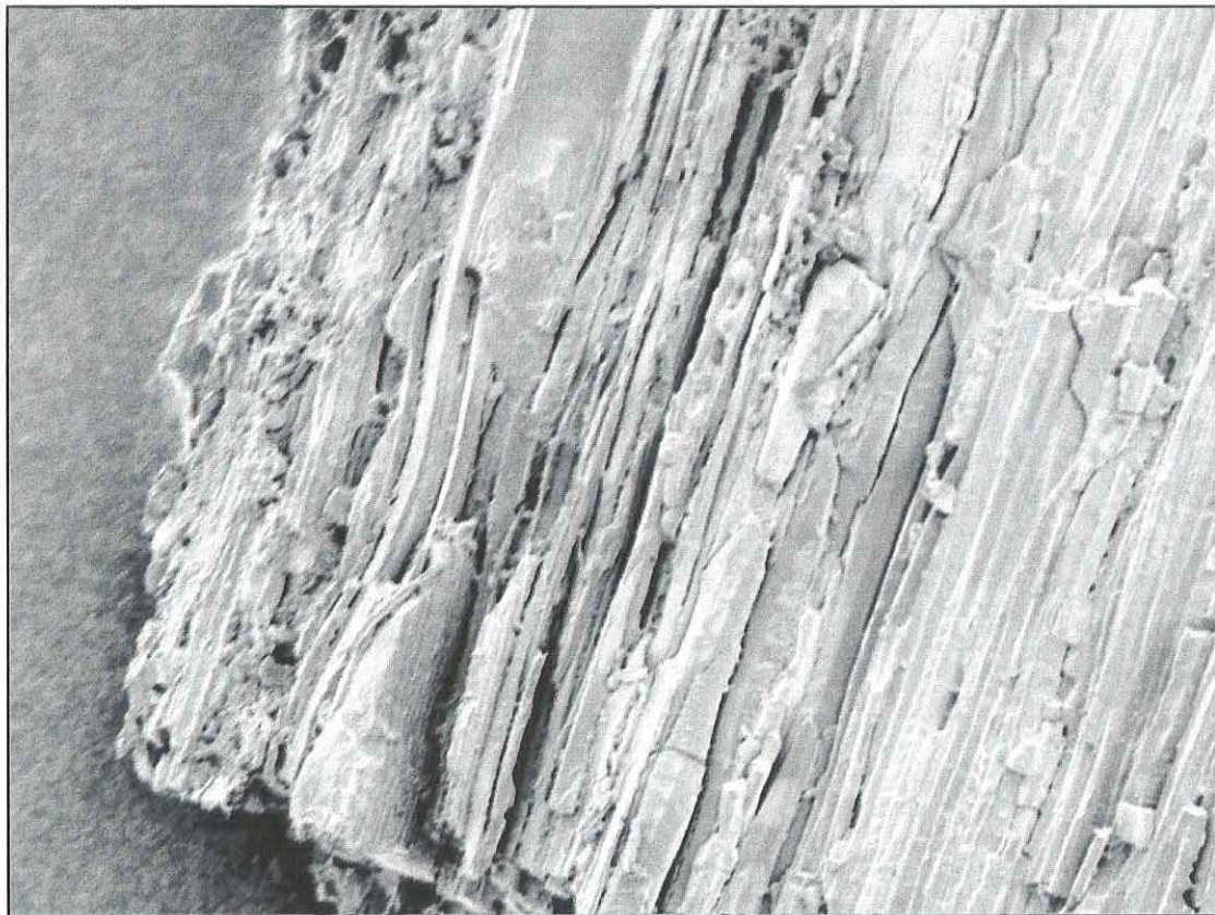
Figure 4. Tangential section of wood from the mouth, note large vessels in the earlywood and ray cells replaced by copper salts, the wood structure has been lost. Mag. around 250x.
