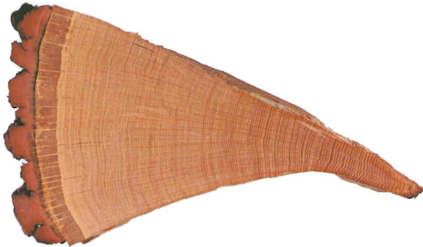
Fig 1. A wedge of oak from a tree felled in 1976. It shows the annual growth rings, one for each year from the innermost ring to the last ring on the outside just inside the bark. The year of each ring can be determined by counting back from the outside ring, which grew in 1976.
