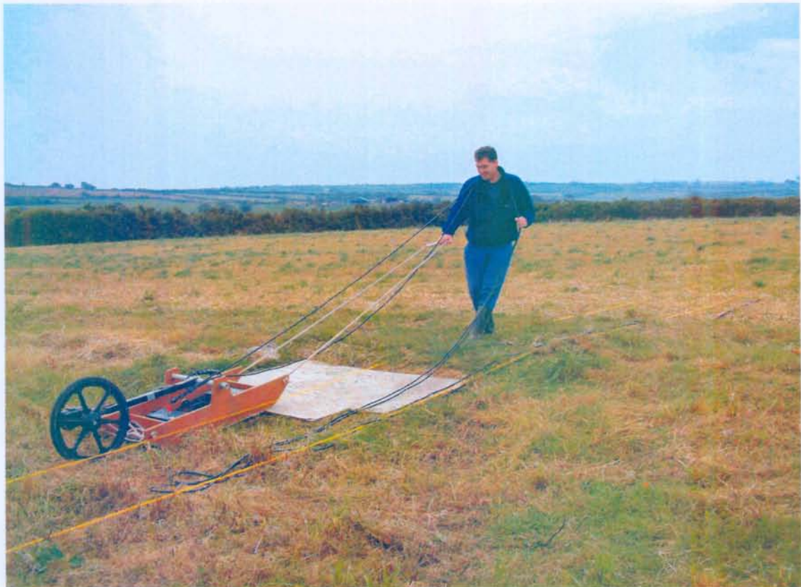
Figure 8 A temporary plywood sheet cover was established over the collapsed void to allow the sledge mounted GPR antenna to pass unhindered over the site.
