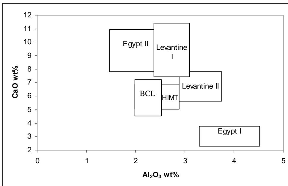
Figure 13: Lime versus alumina for groups of natron glass common in the Mediterranean region in the mid- to late-first millennium AD, identified by Freestone et al, 2002, compared to the adjusted data for the Binchester, Colchester and Lincoln glass samples from this study (BCL group).
