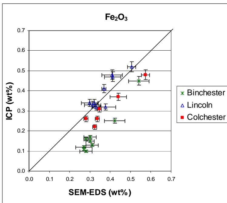
Figure 9: Plot of SEM-EDS data and ICP data for iron oxide
