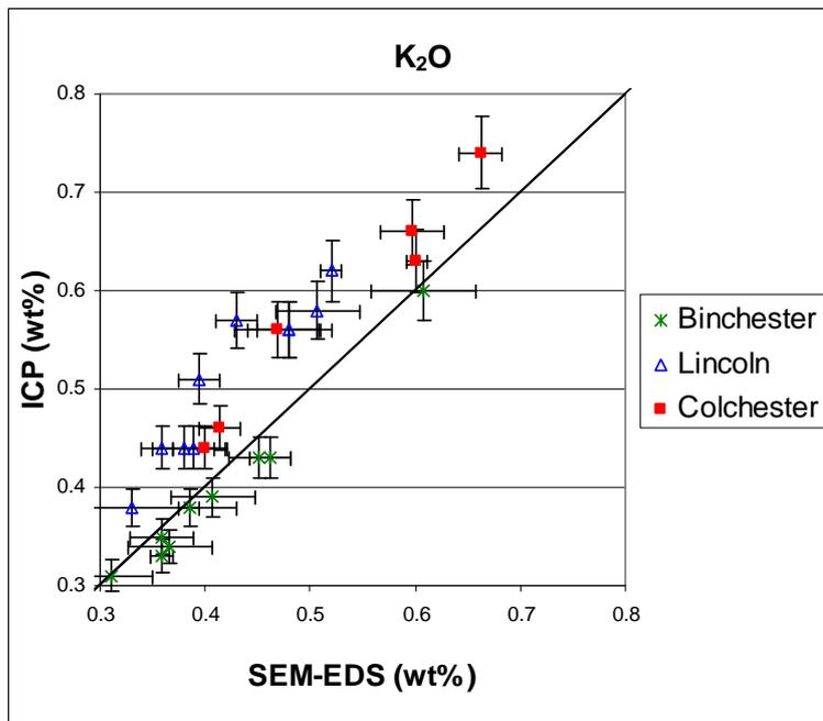
Figure 8: Plot of SEM-EDS data and ICP data for potash
