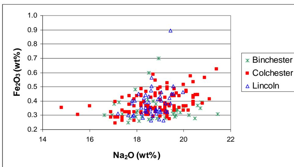
*Figure 10: Plot of adjusted soda and iron oxide ICP data for the Colchester, Binchester and Lincoln glass.*
