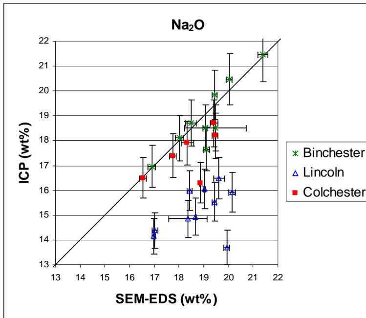
Figure 4: Plot of SEM-EDS data and ICP data for soda
