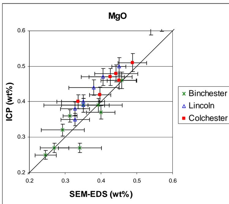
Figure 5: Plot of SEM-EDS data and ICP data for magnesia
