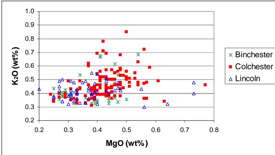
Figure 11: Plot of adjusted magnesia and potash ICP data for the Colchester, Binchester and Lincoln glass.
