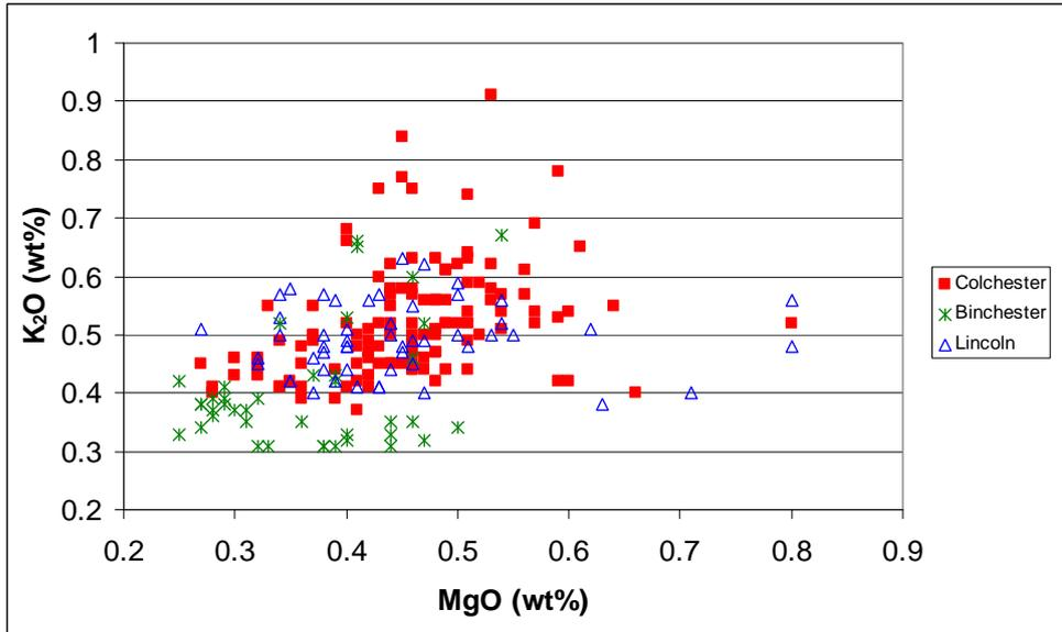
Figure 2: Plot of ICP data for magnesia and potash for the Colchester, Binchester and Lincoln glass
