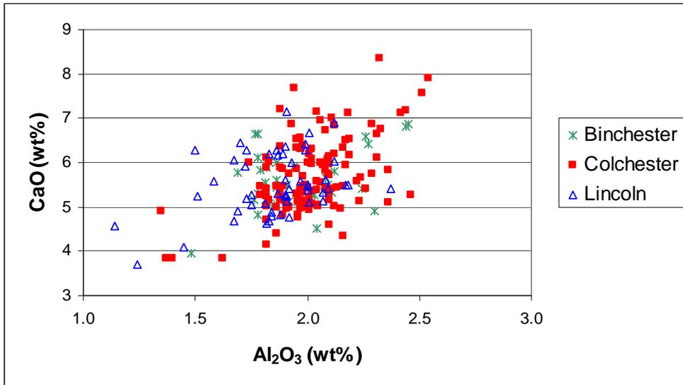
Figure 12: Plot of adjusted alumina and lime ICP data for the Colchester, Binchester and Lincoln glass.
