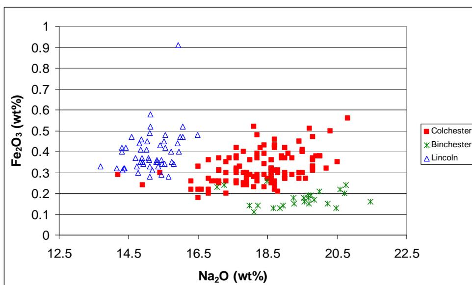
Figure 1: Plot of ICP data for soda and iron oxide for the Colchester, Binchester and Lincoln glass.
