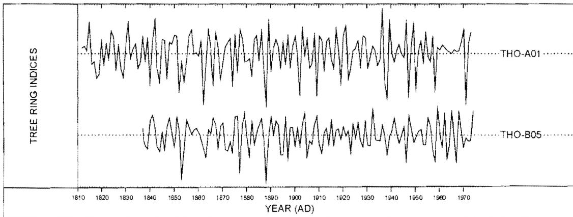
Fig 7. (a) The raw ring-widths of two samples, THO-A01 and THO-B05, whose felling dates are known. Here the ring widths are plotted vertically, one for each year, so that peaks represent wide rings and troughs narrow ones. Notice the growth-trends in each; on average the earlier rings of the young tree are wider than the later ones of the older tree in both sequences.
