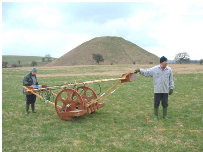
Figure 1 The cart-mounted array of caesium magnetometer sensors in Area 1 with Silbury Hill in the background.
