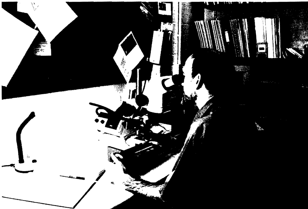
Fig. 3 Measuring ring widths under a microscope. The microscope is fixed while the sample is on a moving platform. The total sequence of widths is measure twice to ensure that an error has not been made. This type of apparatus is needed to process a large number of samples on a regular basis.
