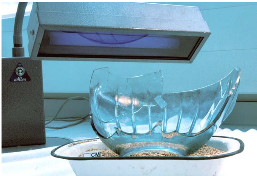
Fig 2 : Cyanoacrylate adhesive curing under UV light
