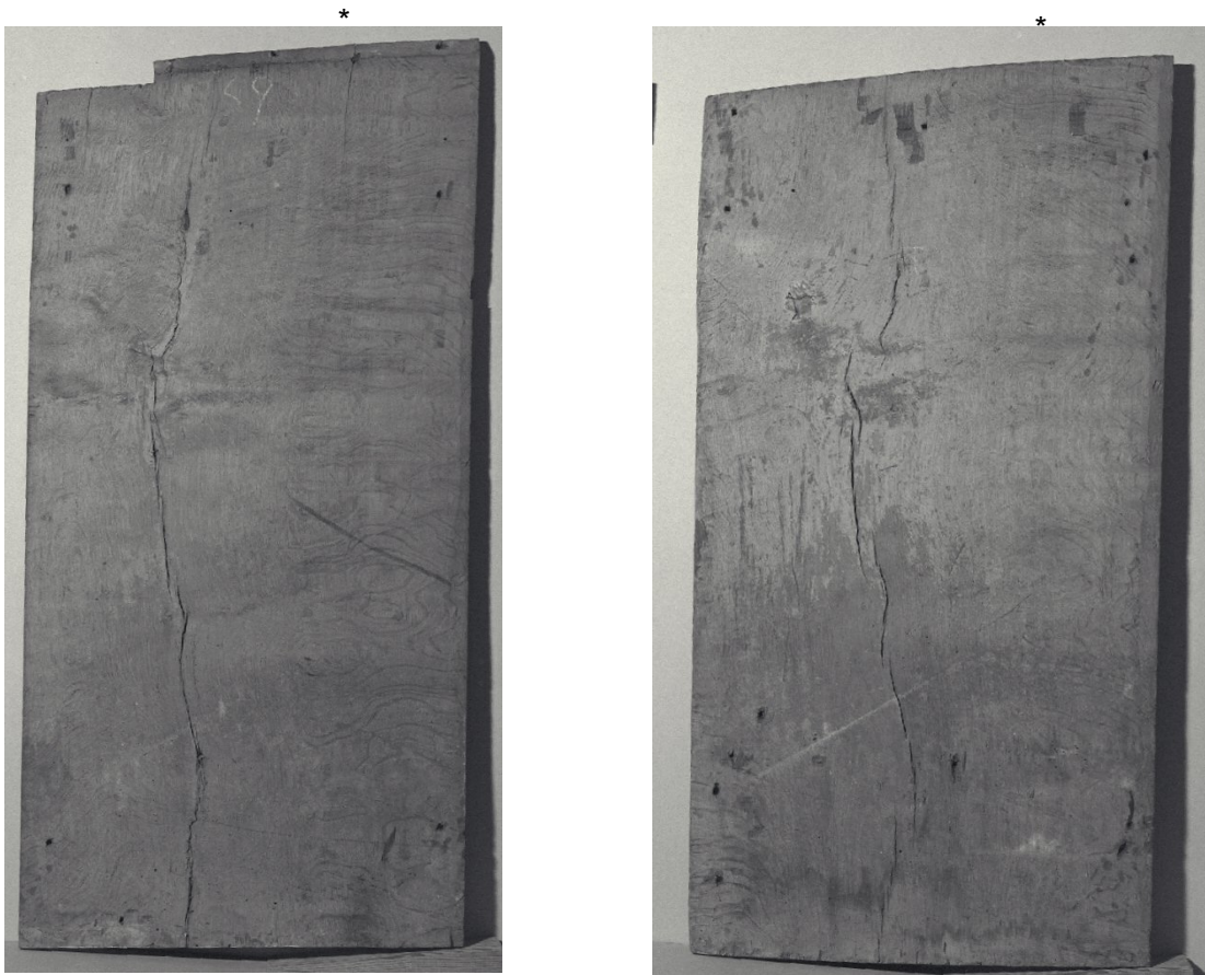
Figure 4 Reverse side of boards 6 (left) and 10 (right) from the Doom panel, Dauntsey Church, Wiltshire. The same knot pattern, the same kink in the centreline, and the same alignment of the grain indicates these were derived from the same length of a single trunk. The exceptionally high t-value between these sequences ( t = 18.58 ) confirms this observation. * marks the measured and dated radii (photographs from the English Heritage Metric Survey Team)
