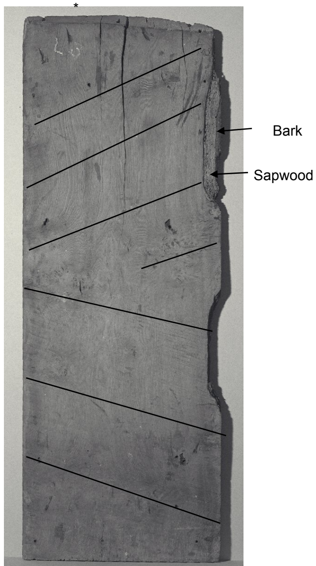
Figure 6 Reverse side of board 3 from the Doom panel, Dauntsey Church, Wiltshire, showing the area of sapwood and bark. The superimposed lines illustrate the angle of the sawing on this board and the adjustment in the alignment as the baulk was turned on the trestle. * marks the measured and dated radius (photographs from the English Heritage Metric Survey Team)
