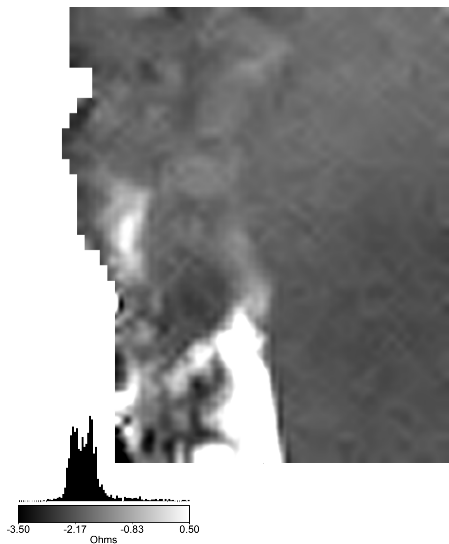
c) 0.5m electrode separation data from a) after subtraction of corresponding reading from 1.0m separation data from b). The latter was first corrected for the difference in mobile electrode separation. The result accentuates near surface anomalies.
