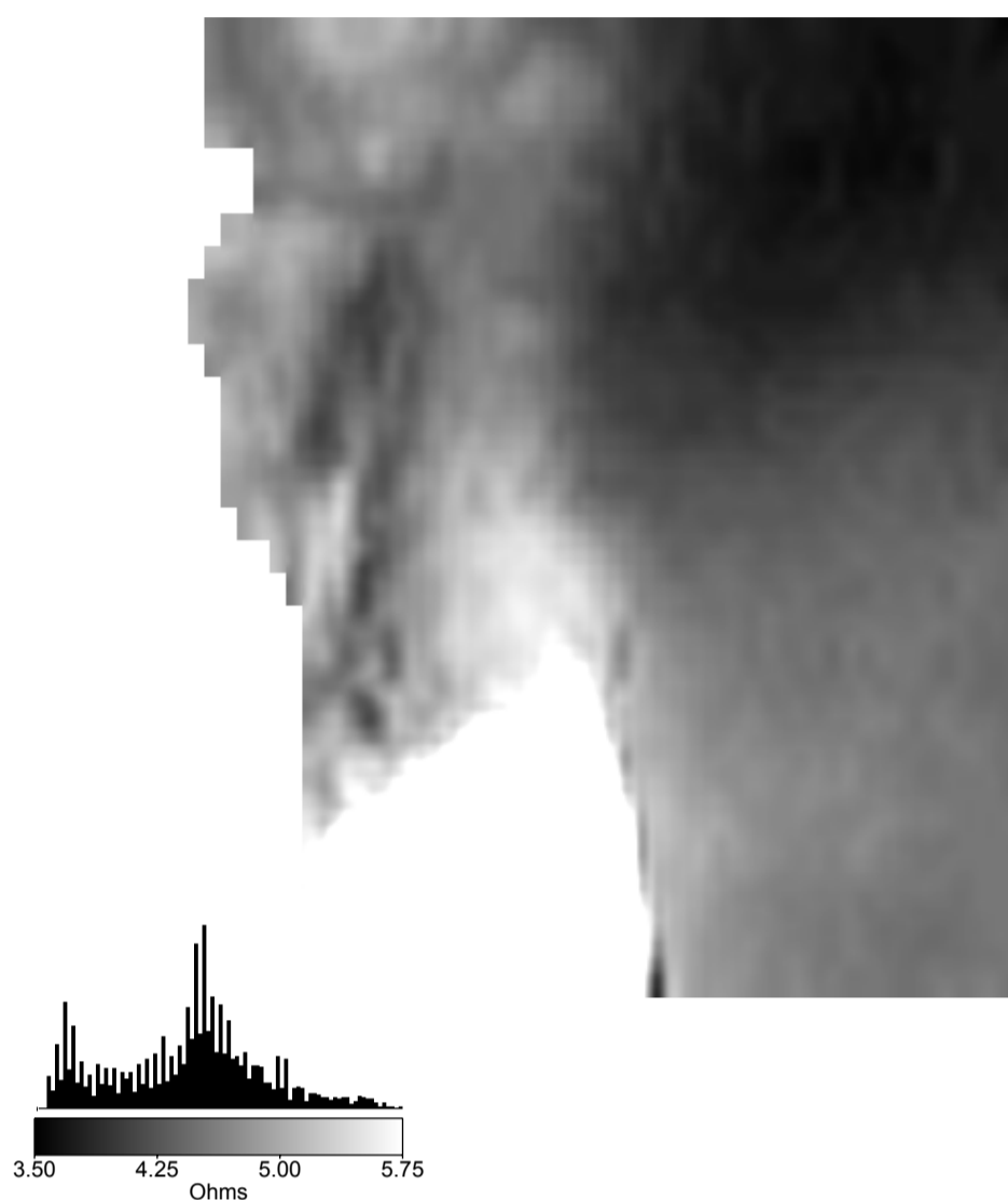
b) Greyscale plot of 1.0m mobile electrode data after filtering with local neighbourhood directional smoothing algorithm.
