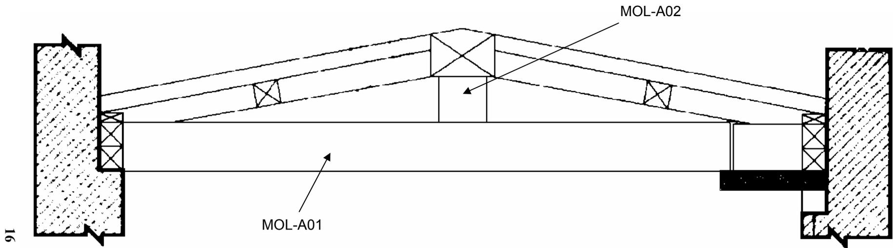
Figure 6: Roof truss, north truss, showing the location of samples MOL-A01 and MOL-A02 (Hockley and Dawson)
