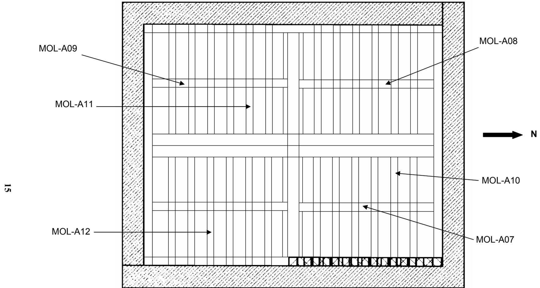
Figure 5: Plan of roof structure, showing the location of samples MOL-A07–12 (Hockley and Dawson)
