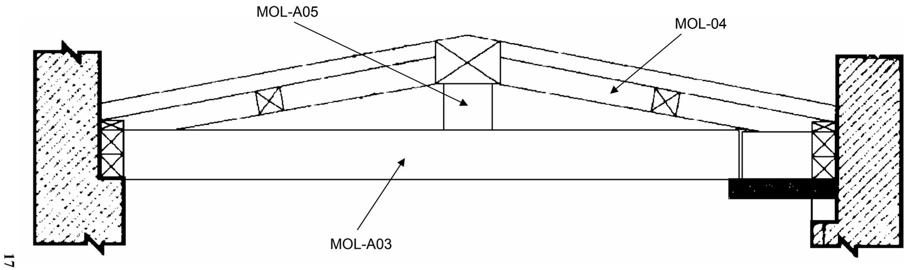
Figure 7: Roof truss, mid truss, showing the location of samples MOL-A03–5 (Hockley and Dawson)
