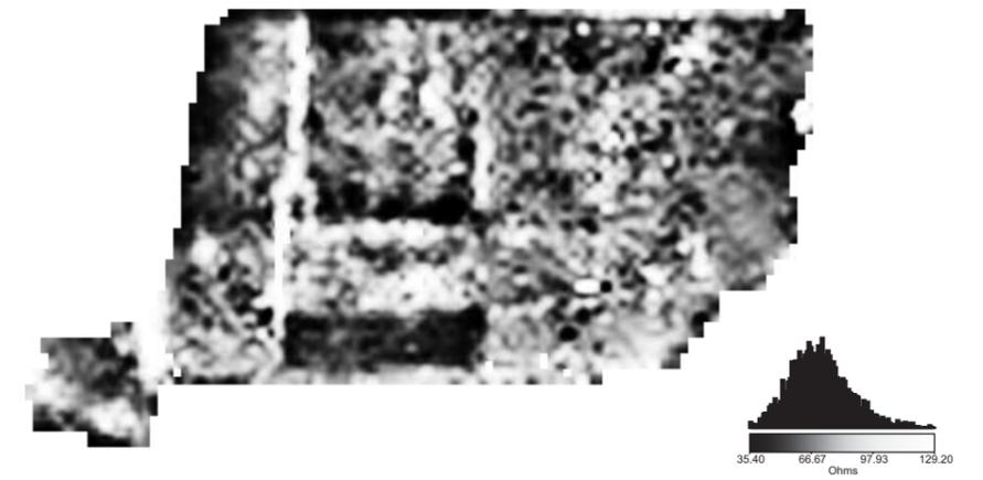
D) Traceplot of resistance data at one metre probe spacing.
