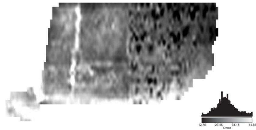
F) Greyscale plot of contrast enhanced resistance data at one metre probe spacing.
