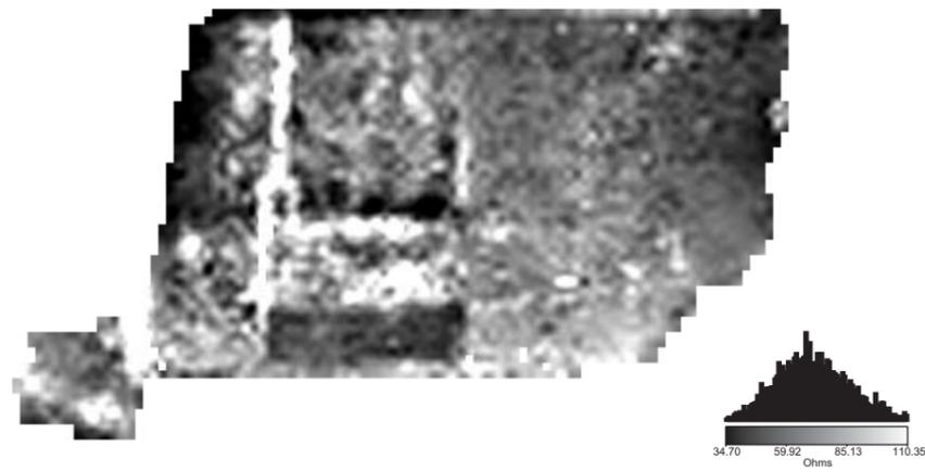
C) Greyscale plot of contrast enhanced resistance data at half metre probe spacing.
