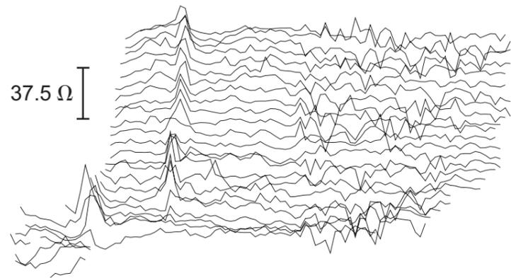
E) Linear greyscale plot of resistance data at one metre probe spacing.
