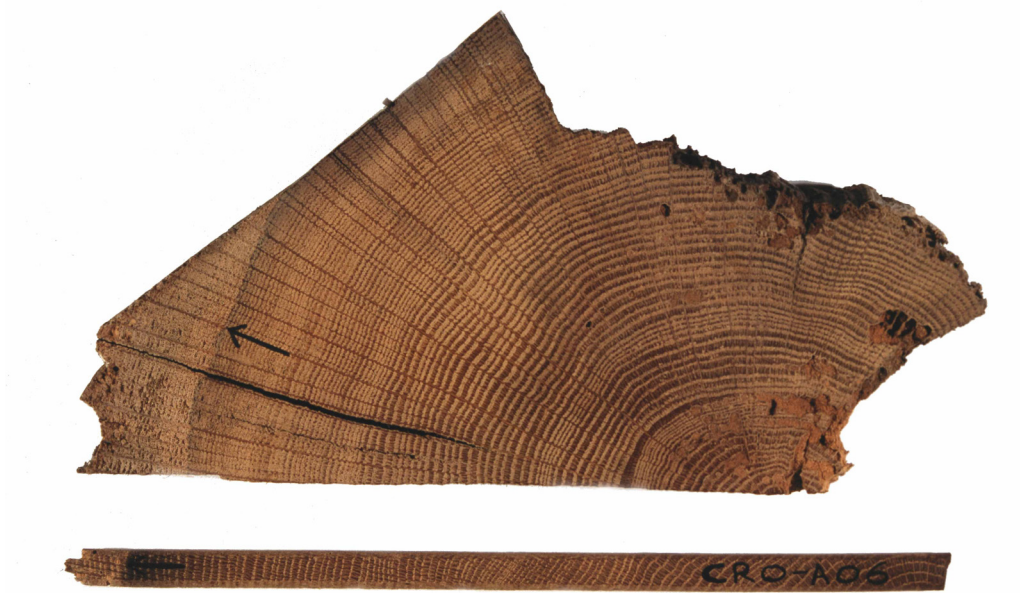
Figure 2: Cross-section of a rafter showing the presence of sapwood rings in the left hand corner, the arrow is pointing to the heartwood/sapwood boundary (H/S). Also a core with sapwood; again the arrow is pointing to the H/S. The core is about the size of a pencil.
