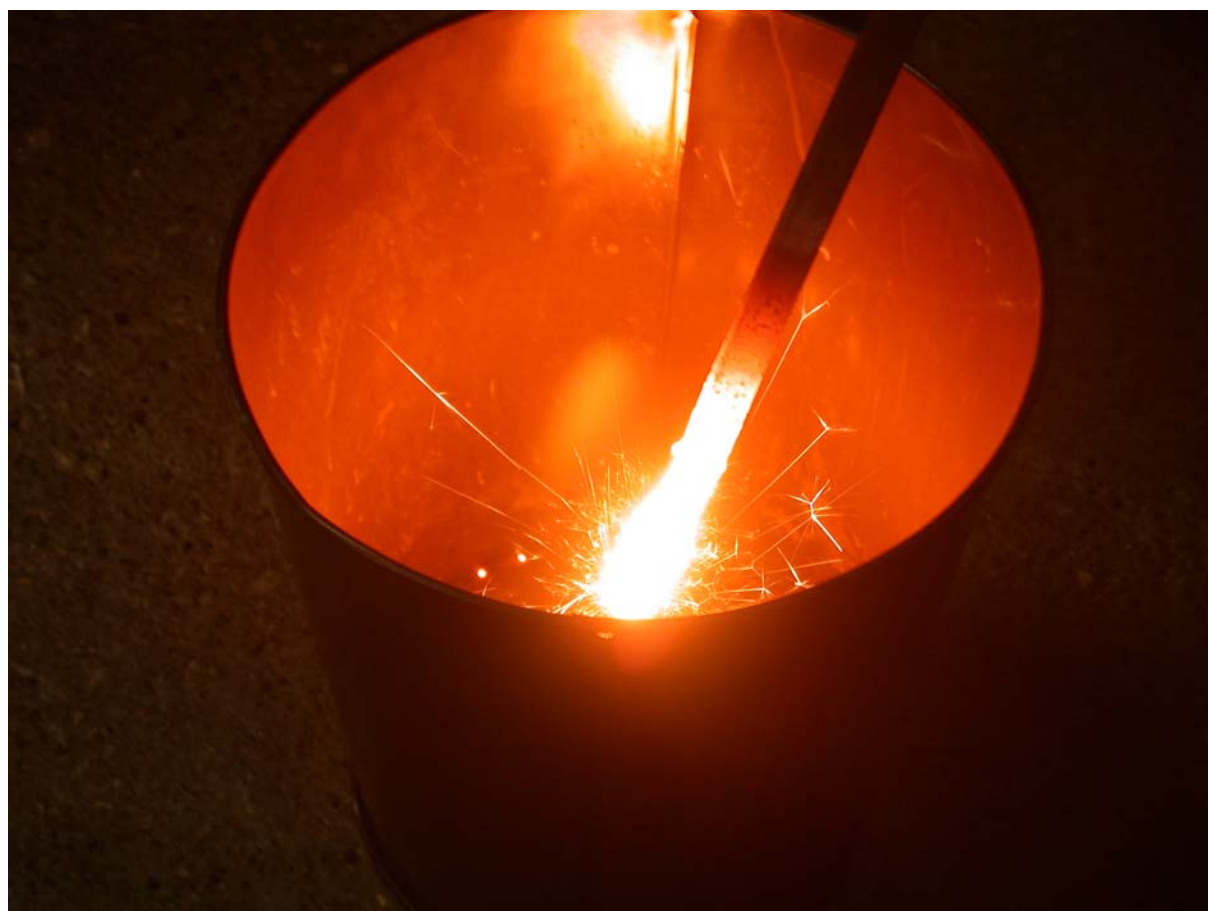
Figure 12. An over-heated bar of iron with the spheroidal material collected in a container
