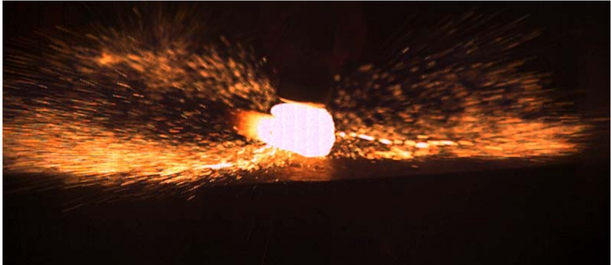
Figure 16. Welding experiment 16. Still from the high-speed digital camera 11 frames after the impact
