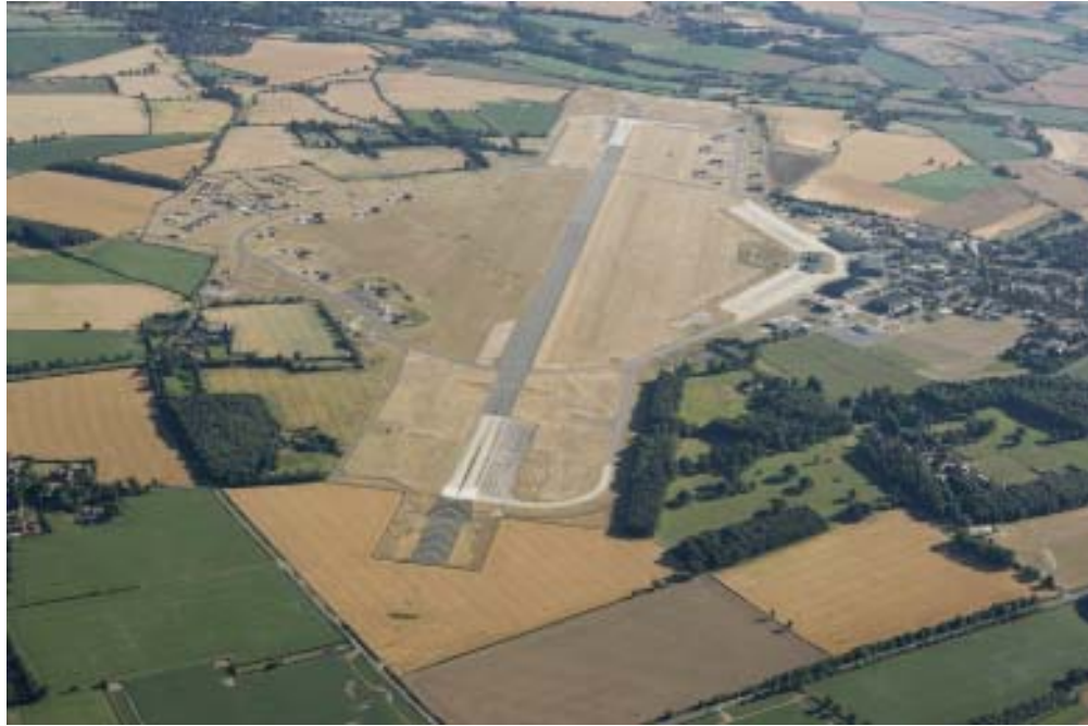
Figure 248 RAF Coltishall viewed from the north east looking along runway 22. To the right are the airfield's domestic and technical area, including a control tower four large hangars. To the left are the wartime bomb stores and post war missile storage area. The original flying field was grass during the war this reinforced by steel matting and after the war in anticipation of the introduction of jet fighters replaced by a concrete runway and taxiways. In the mid-1950s the dispersed concrete blast protection walls were built to protect aircraft against low level strafing attacks. (c) English Heritage NMR 24369/009
