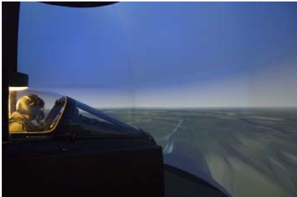
Figure 177 Jaguar Flight Simulator building, training cockpit and terrain image projected inside the hemisphere. (c) English Heritage DP027168
