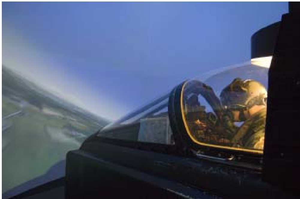
Figure 181 Jaguar Flight Simulator building, training cockpit and terrain image projected inside the hemisphere. (c) English Heritage DP027180
