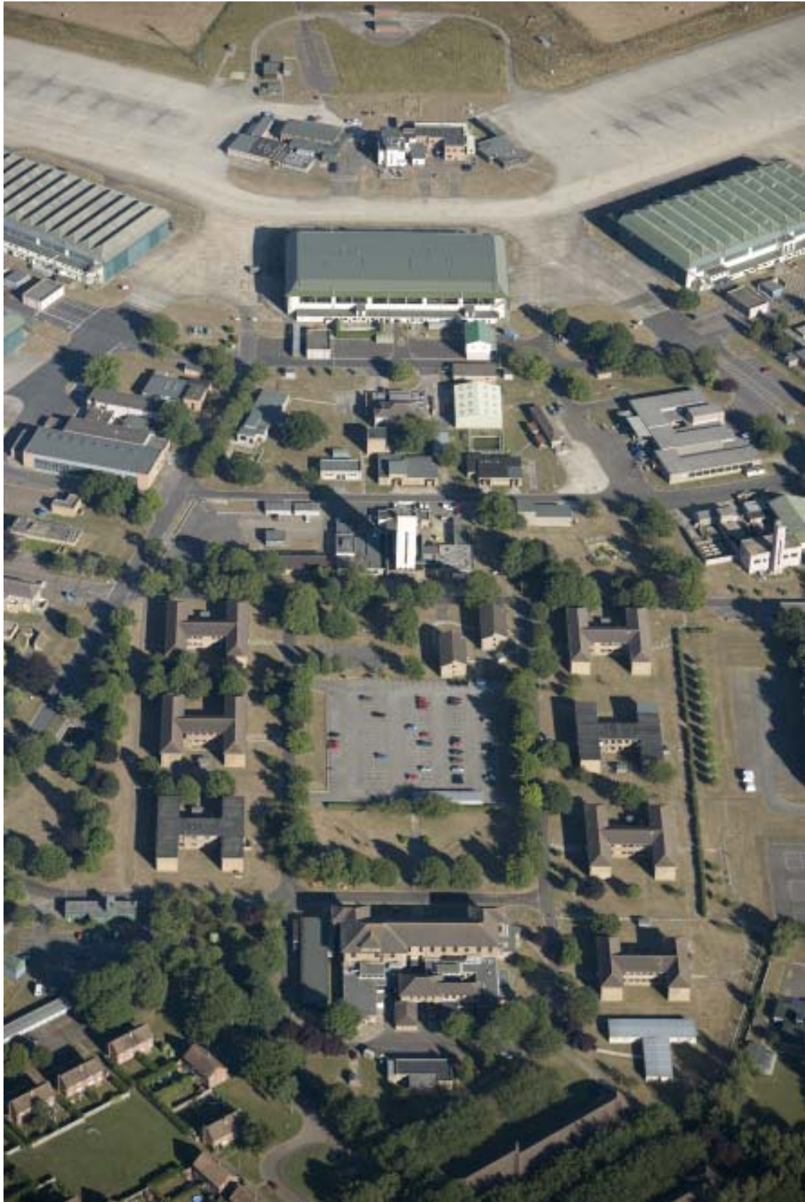
Careful consideration was given to the landscape design of the RAF's 1930s permanent airfields. This is evident in the careful symmetry of the roads and the use of trees to create a pleasant working and living environment. To the top is part of the airfield's technical area, including the watch office, hangars, stores and workshops. In the centre is the tall water tower, the H-shaped 1930s barracks and at the bottom the large airmen's institute. © English Heritage NMR 24369/037
