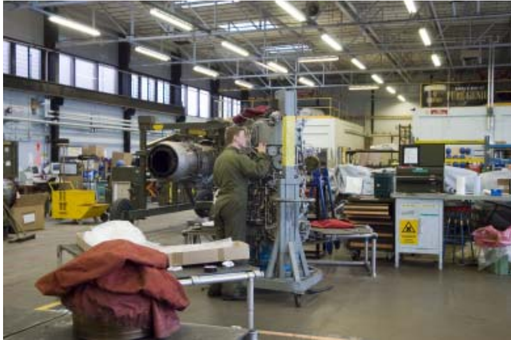
Figure 156 Propulsion and Aircraft Components Flight (PACF) Adour Engine Assembly Facility. Friday, 24 March 2006 work underway on the assembly of the last Rolls-Royce Turbomeca Engine built at RAF Coltishall, engine number 1229E. (c) English Heritage DP029249
