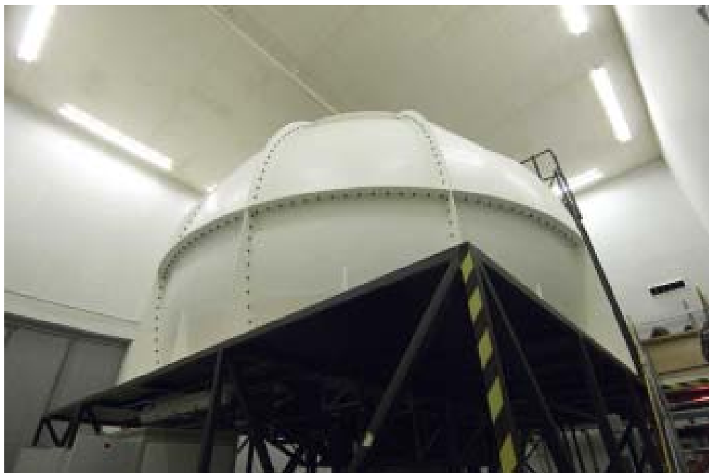
Figure 173 Jaguar Flight Simulator building, rear of fibreglass hemisphere into which images of the moving terrain were projected. (c) English Heritage DP027195
