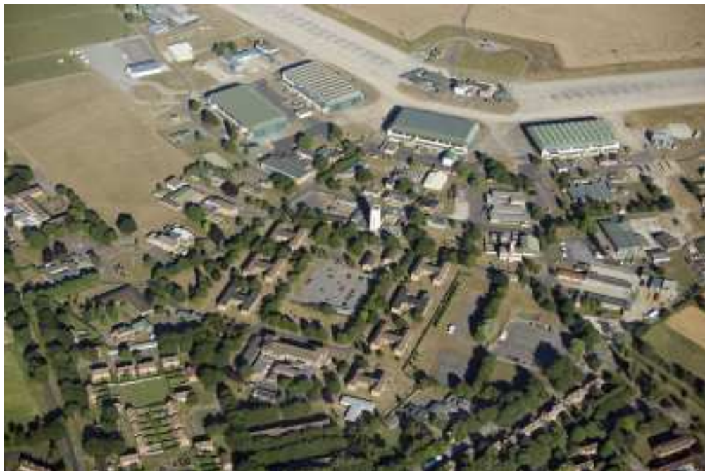
Figure 2 RAF Coltishall, from southwest. To the top is the Watch Office, or Control Tower, and four C type hangars, between them and the H-shaped barrack blocks is the technical area, including the parachute packing building, engine maintenance building and stores. (c) English Heritage NMR24369/038
