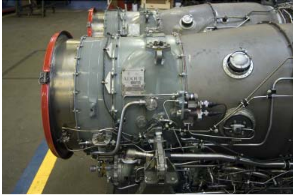
Figure 155 Propulsion and Aircraft Components Flight (PACF) Adour Engine Assembly Facility, detail of Rolls-Royce Turbomeca engine 1220E. (c) English Heritage DP029252
