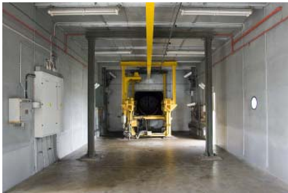
Figure 163 Uninstalled Engine Test Facility (UETF), test chamber looking towards the mouth of the detuner, which reduced the noise during test firing. (c) English Heritage DP027325
