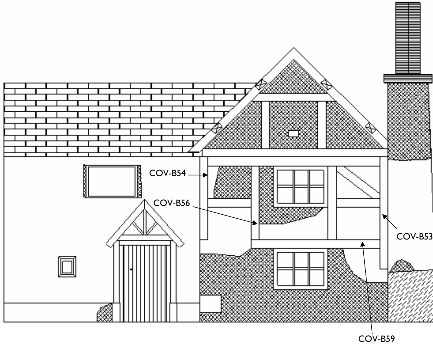
Figure 12: Cromwell Cottage; east elevation, showing the location of samples COV-B53, COV-B54, COV-B56, and COV-B59 (Frank W Haywood & Associates)
