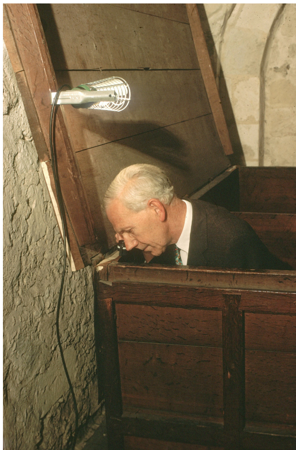
Figure 7: Dr John Fletcher measuring ring sequences of Greater Treaty Chest (D Haddon-Reece)
