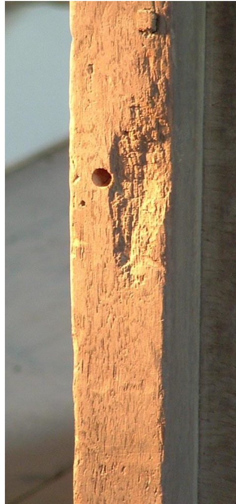
Figure 46: Micro-bore hole (8mm diameter) and core (M Bridge)
