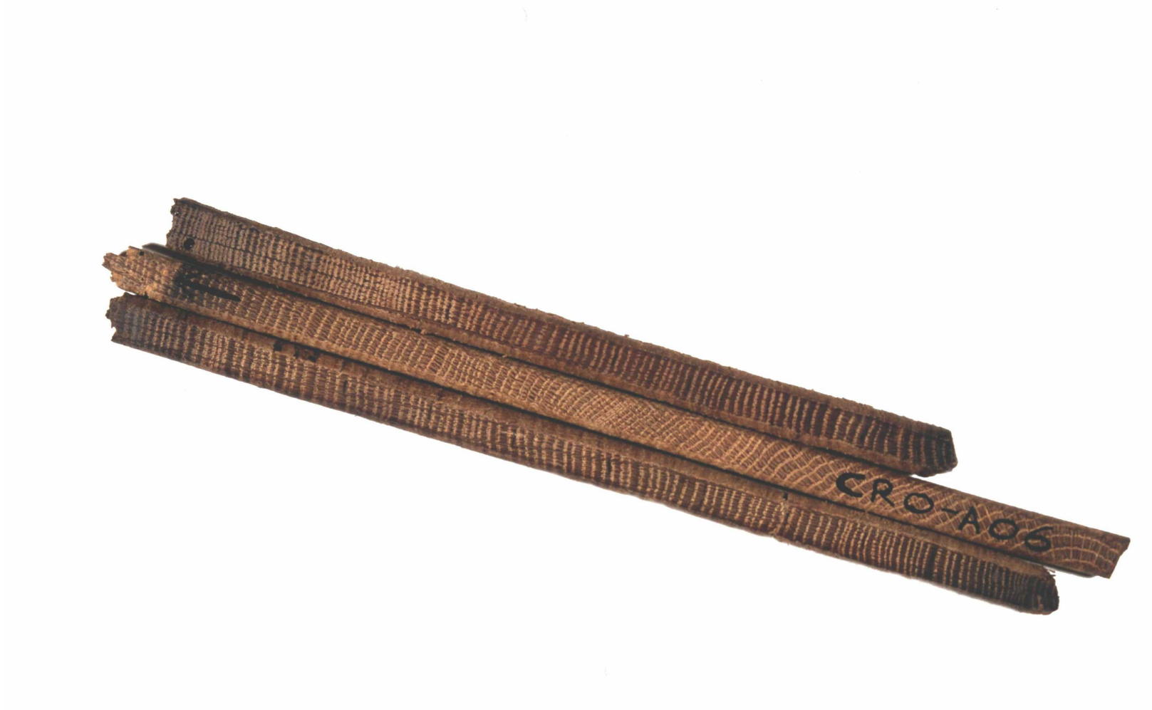
Figure A4: Three cores from timbers in a building. They come from trees growing at the same time. Notice that, although the sequences of widths look similar, they are not identical. This is typical
