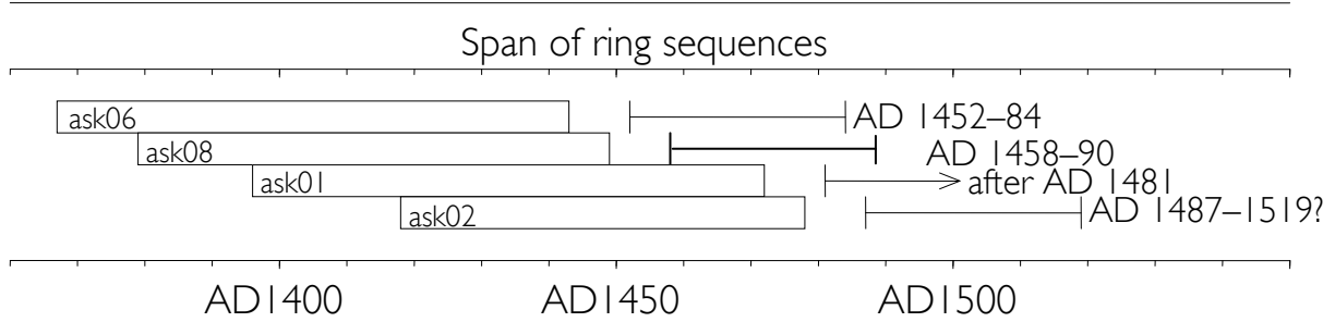
Figure 3: Bar chart showing the relative positions of overlap of the dated timbers along with their derived felling date ranges
