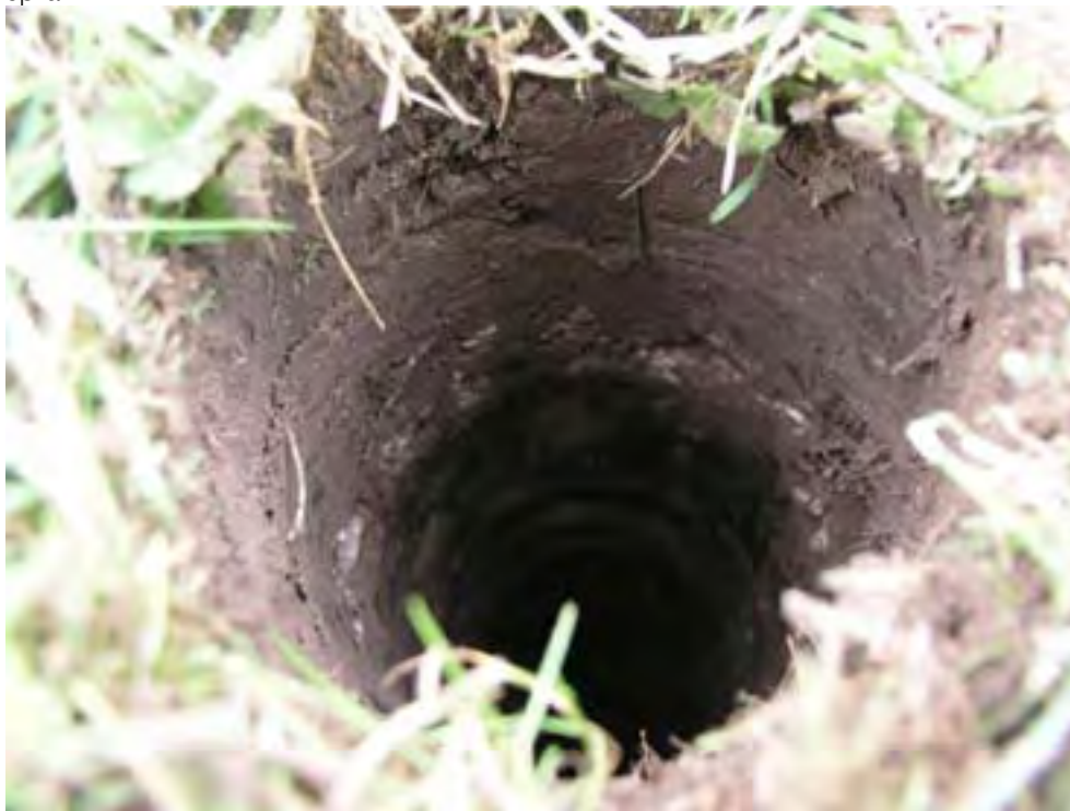
Figure 15. View down Hole 10 after extraction of the core showing limestone chippings at 15 – 20 cm depth.
