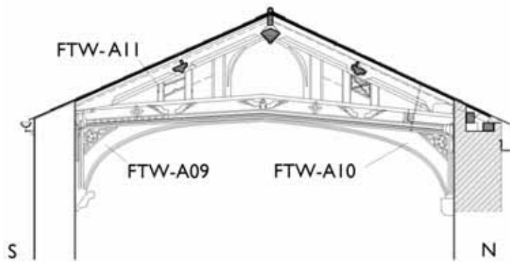
Figure 11: East elevation of principal truss 5 (based on truss 11), showing the location of samples FTW-A09–11 (Freeland Rees Roberts Architects)
