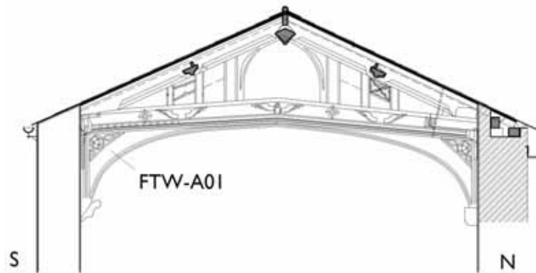
Figure 7: East elevation of principal truss 1 (based on truss 11), showing the location of sample FTW-A01 (Freeland Rees Roberts Architects)
