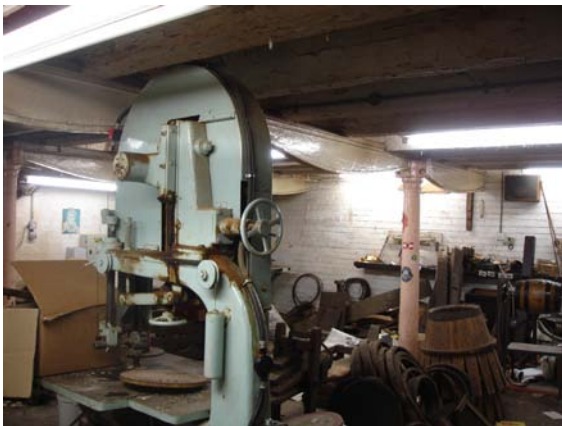
Figure 69 The ground floor of the cooperage. Note the 'fish-bellied' beams. DP070427.
