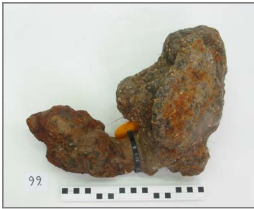
Figure 3: Type 3. Find no. 99 - concretion containing a hook with solid core and corroded outer edge
