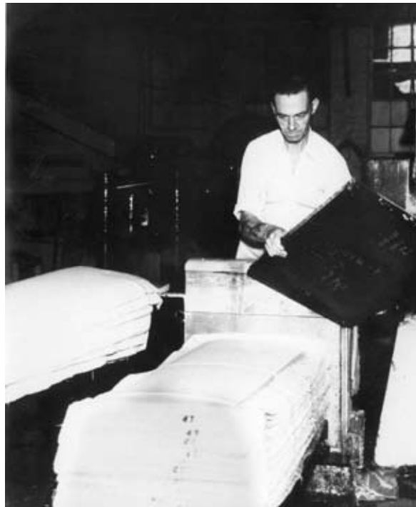
Figure 79: Undated (c.1950s) view of coucher at Laverstoke. He is building up a 'post' of alternating layers of felt and paper (photograph supplied by Nick Pearson).
