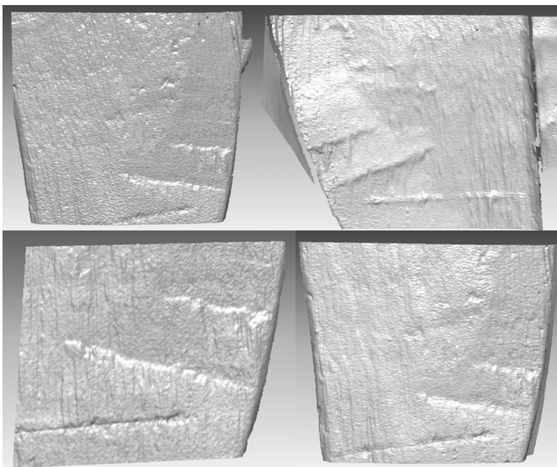
Fig 15: Visual comparison of the scans confirms a progressive softening of the sharpened edges present in the pre-treatment timber (clockwise from top left: pre-treatment timber, silicone mould, post-treatment timber, plaster cast)
