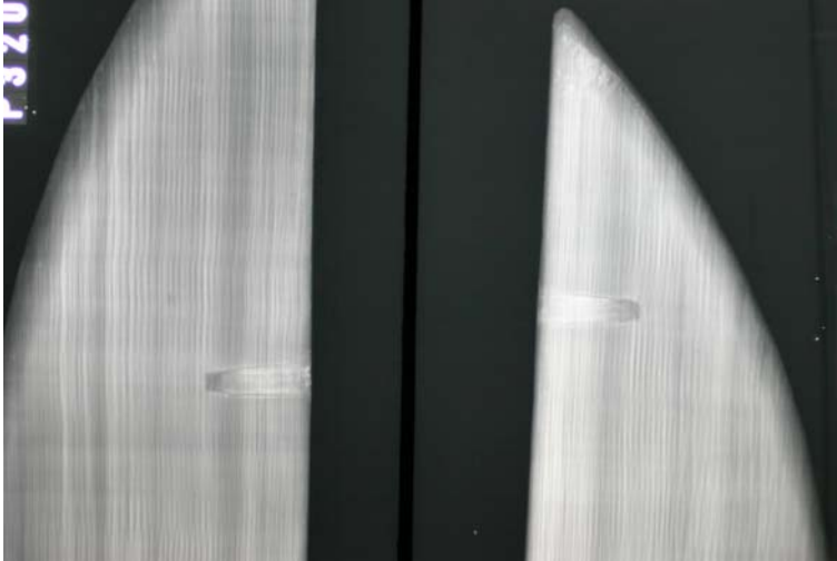
Fig 9: X-radiograph of dowels within the head piece 2255
