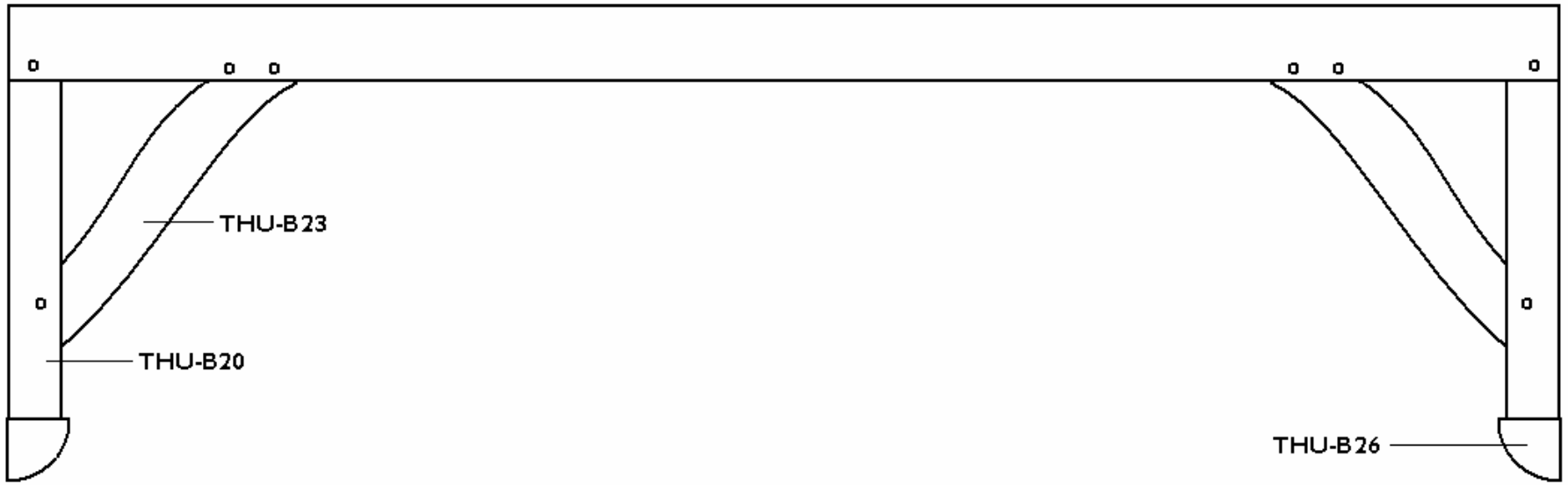
Figure 9: Lower in-situ timbers; sketch of west truss, showing the location of samples THU-B20, THU-B23, and THU-B26
