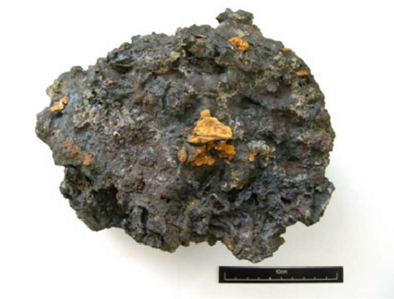
Fig 2: Top surface of fragment SCI. Note the yellowy orange corrosion which may have been in contact with the bloom.
