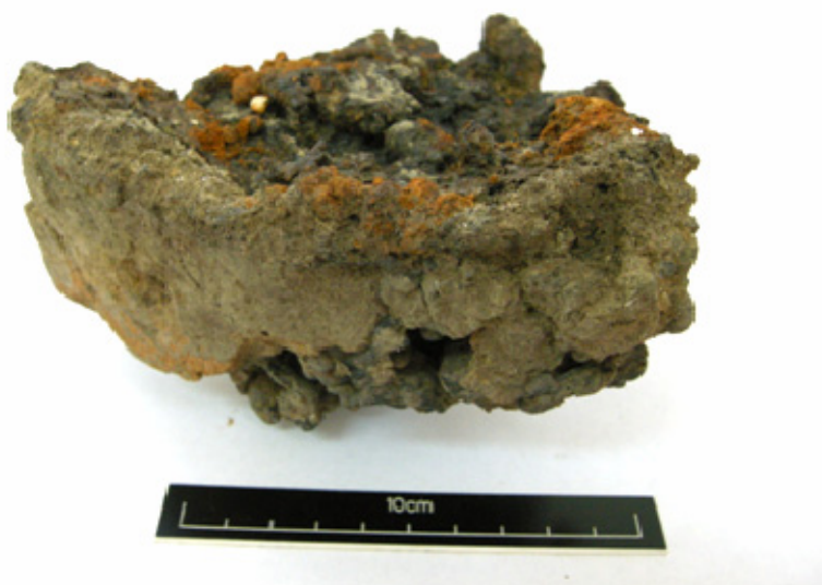
Fig 4: Rounded clay side of fragment SC4. Note the orangey corrosion which may be the result of contact with the iron bloom.
