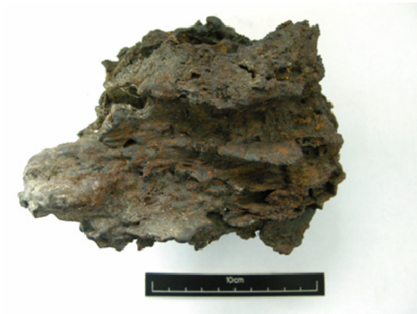
Fig 5: Parallel charcoal impressions on a slag block fragment.
