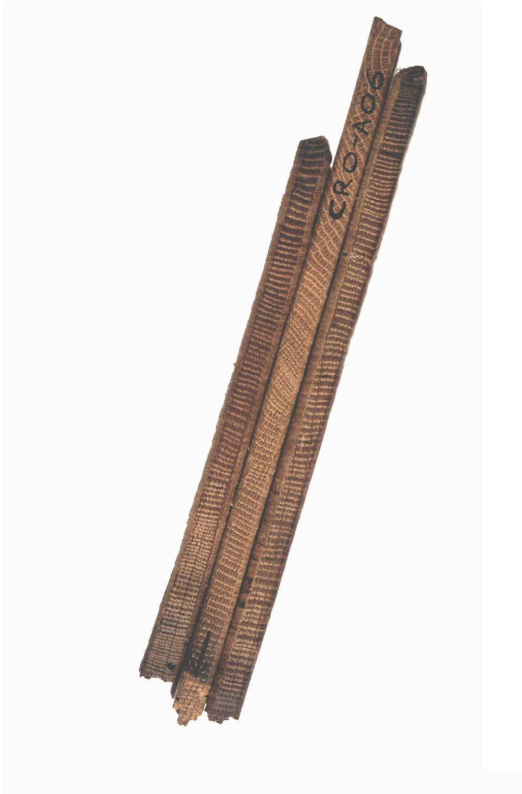
Figure A4: Three cores from timbers in a building. They come from trees growing at the same time. Notice that, although the sequences of widths look similar, they are not identical. This is typical
