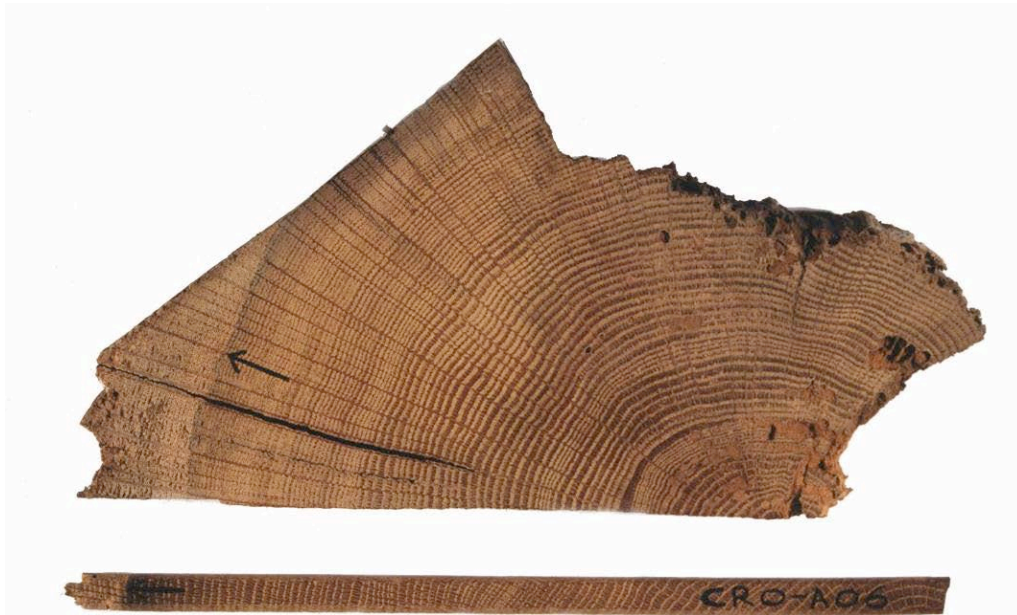
Figure A2: Cross-section of a rafter, showing sapwood rings in the left-hand corner, the arrow points to the heartwood/sapwood boundary (H/S); and a core with sapwood; again the arrow is pointing to the H/S. The core is about the size of a pencil
