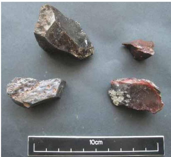
*Figure 19: Glassy copper slag (sample #2 is top left)*
