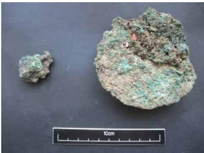
*Figure 18: Copper alloy lump, left, and right, sample #5, a hemispherical mass of leaded bronze*
