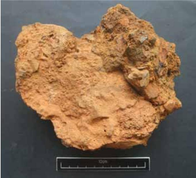
Figure 13: Plan view of sample #10, a large mass of dense fayalitic slag with adhering hammerscale and concretions.
