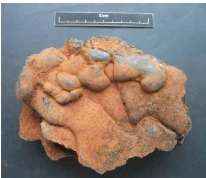
*Figure 4: Top view of flowed fayalitic slag from dry puddling (#11)*
