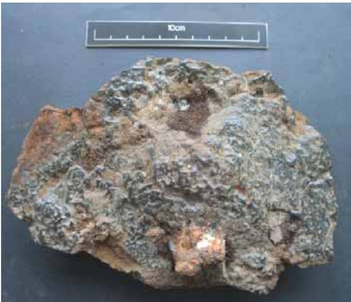
*Figure 6: Underside view of flowed fayalitic slag from an iron conversion process (#11)*
