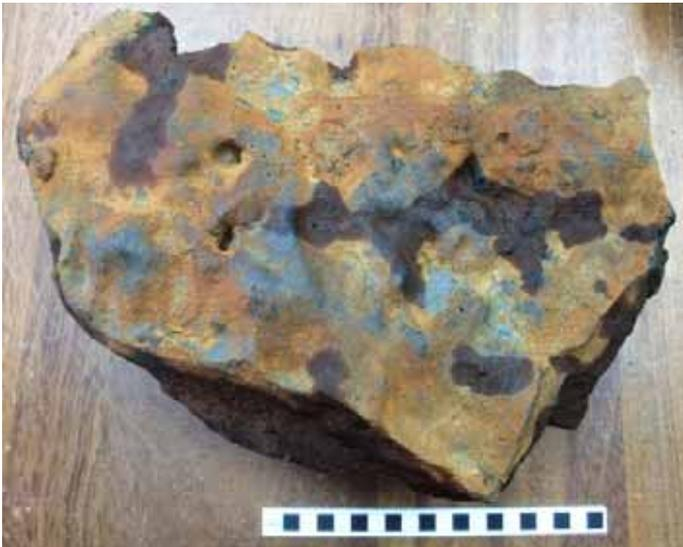
*Figure 11: Upper surface of a large mass of puddling slag adhered to the hearth lining (sample #67)*
