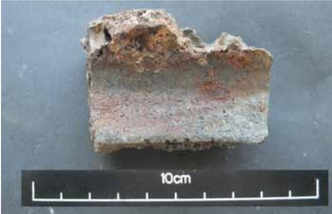
*Figure 7: Plan view of sample #18, which probably derives from refining*
