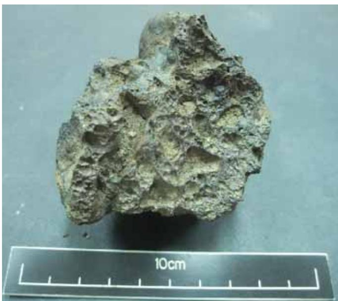
*Figure 15: Bubbly fayalitic slag sample #43*
