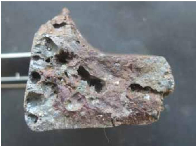
*Figure 8: Side (bottom) view of sample #18, which probably derives from refining*
