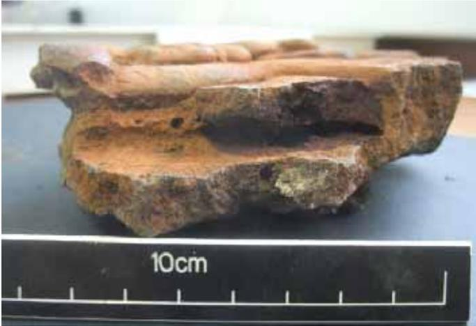
*Figure 5: Side view of flowed fayalitic slag from dry puddling (#11)*
