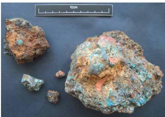
*Figure 16: Bubbly fayalitic slag with green staining from copper corrosion products and adhering orange-fired fragments of ceramic (sample #6)*
