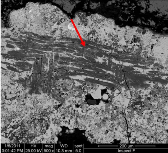
Fig 11. Crystalline phase 1c in lith41.
