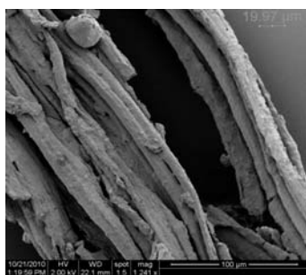
Figure 9: SEM image of sample 3, round fibres from glass vial.
